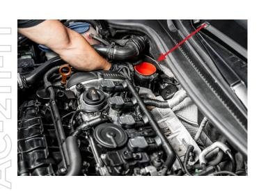
Attach the turbo silicone hose to the turbo inlet and tighten the clamp.
