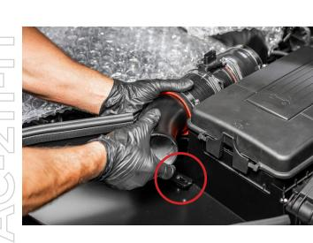
The other side attaches with the intake inlet. Please note that the screw slot on the intake inlet is intended to connect to the intake box.
