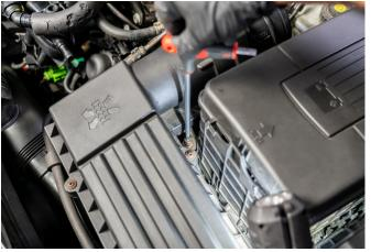
Remove the airbox bracket bolt behind the airbox.
