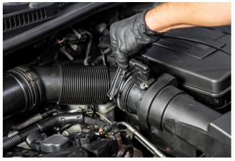
Use your pipe clamp removal tool to release the OEM plastic intake pipe from the MAF housing.
