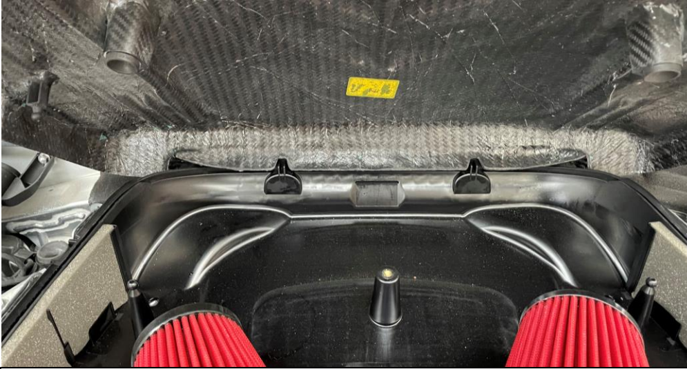
44. Take the carbon lid and push the rear tabs into the slots on the back of the airbox base.
