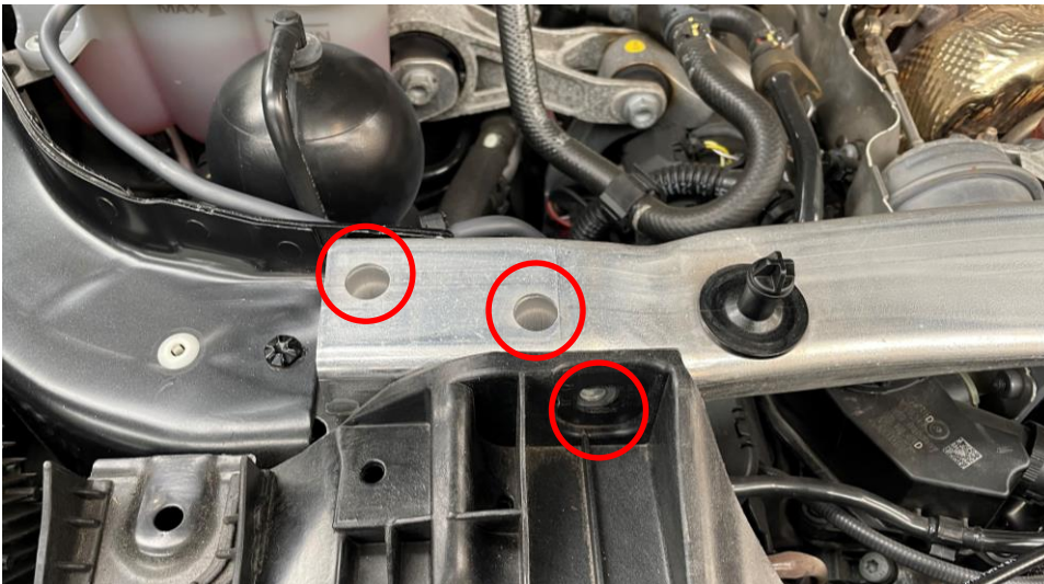
11. Remove the 3 x T30 screws on each side of the strut brace circled in red. There may also be an electrical plug attached to the brace depending on the SUV model. Carefully remove any connectors from the brace. Remove the brace from the engine bay.
