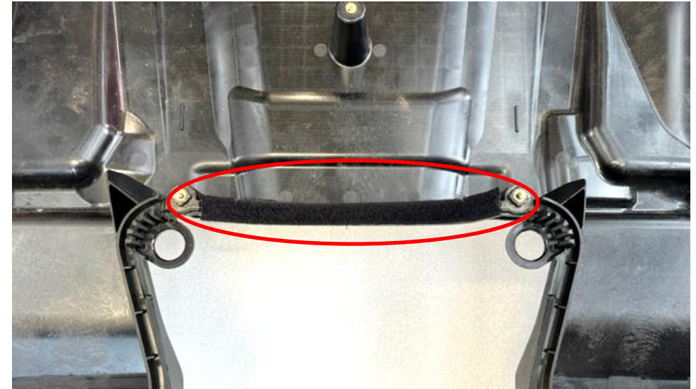
39. Remove the backing and stick it as shown onto the airbox where the collector will sit. This will protect the carbon.
