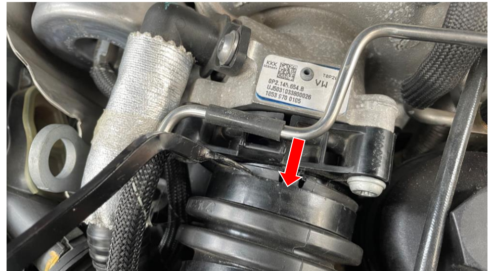
12. To gain easier access to the screws holding the turbo inlets in place, the main body of the inlets can be separated from the flanges. Carefully push the plastic ring shown, away from the turbo flange. Use a lever bar or flat head screwdriver. This releases the body of the inlet – see next photo.
