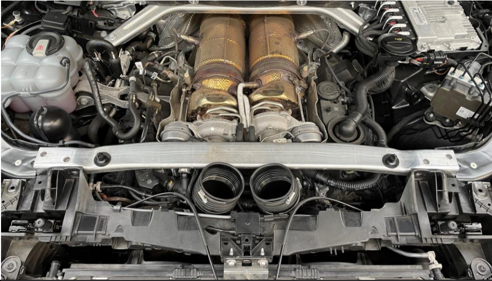
32. Re-fit the strut brace. Secure with the 3 x T30 screws each side. Re-attach any electric connectors (if applicable) to the brace.
