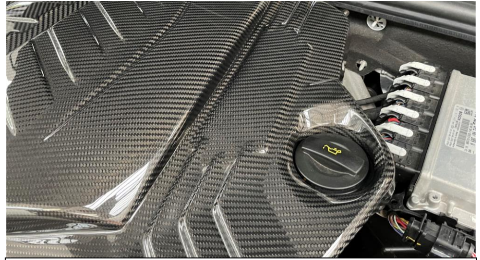
45. As you lower the lid – adjust the oil filler cap so that it sits correctly.
