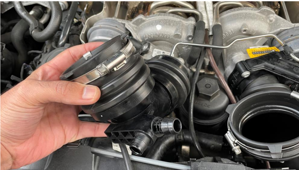
15. The left inlet removed.
