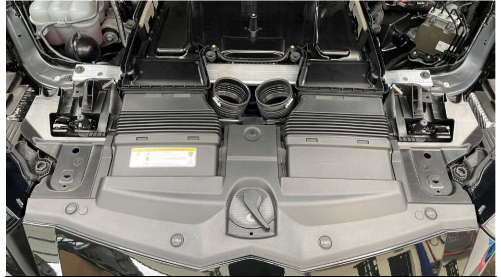
37. Reinstall the front panel and air ducts to the airbox. Secure the panel with the OE clips and also reinstall the hood release lever. It should click into place.
