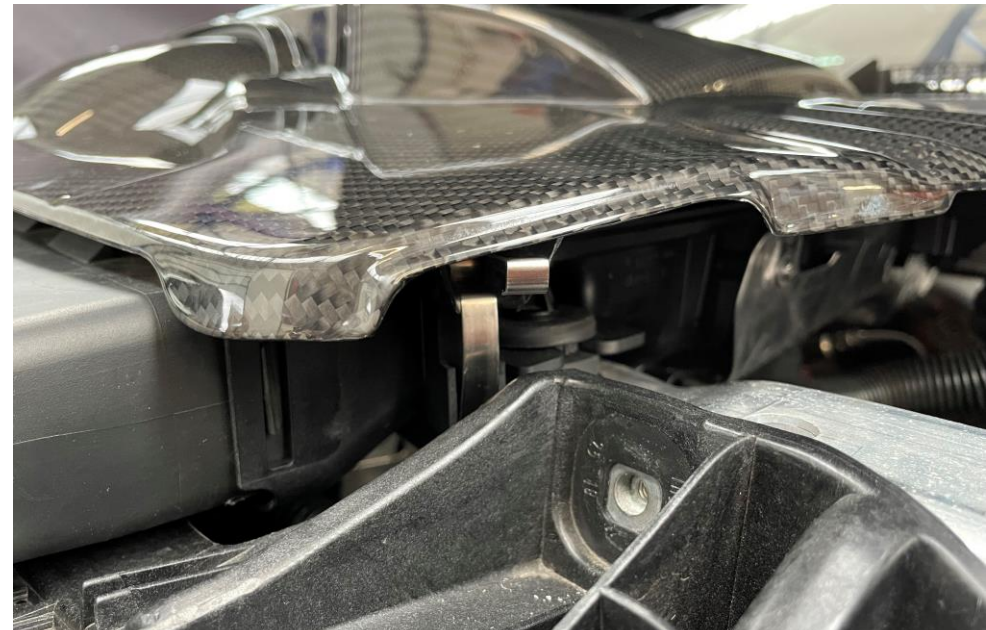
47. Secure the lid with the 2 metal clips on each side at the front.
