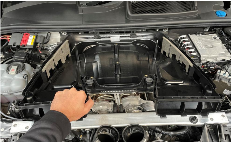
34. Re-install the base of the airbox. Start by pushing it onto the rear mounts shown in the last step. The airbox has rubber grommets which locate onto those mounts.
