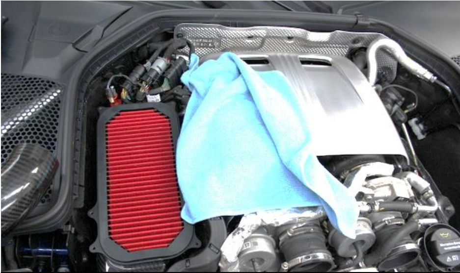
21. Install the filter - make sure it is seated properly all around the flange on the airbox. Place a cloth over the metal engine cover to protect it for the next step.
