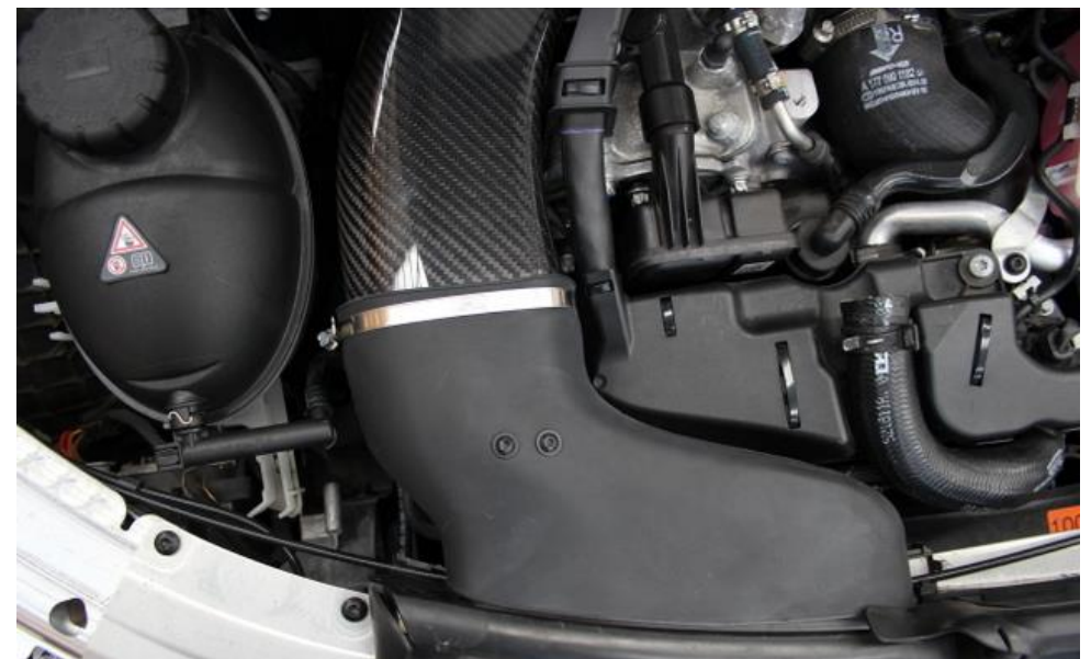
20. The rubber duct should sit as far forward as possible as shown. Once in place tighten the clamp around the carbon – do not over tighten this. It only needs to be finger tight.
