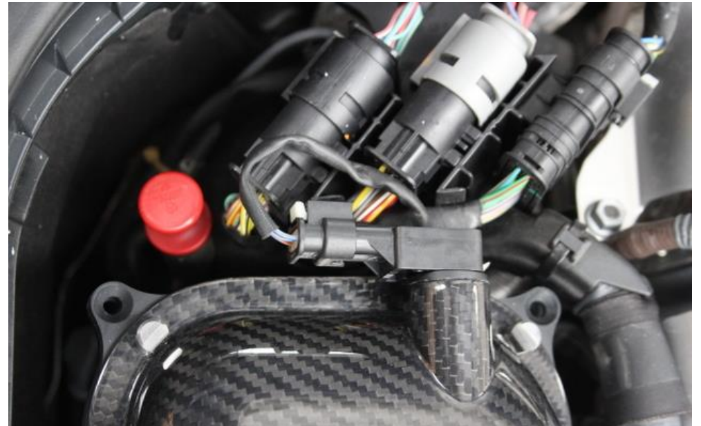
28. Install the MAP sensor plug. Make sure it is fully installed and the locking tab is pushed back in.
