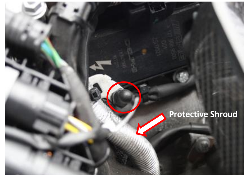
16. The rubber needs to locate onto this mount at the back of the engine. Please rotate the mount on the airbox so that it lines up with the silver protective loom shroud shown.
