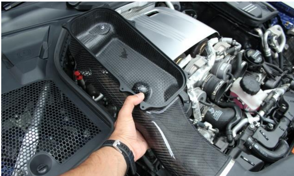
15. Starting with the left side we will install the base first. Before installing please see next step. The rubber mount at the back of the airbox needs to be lined up.
