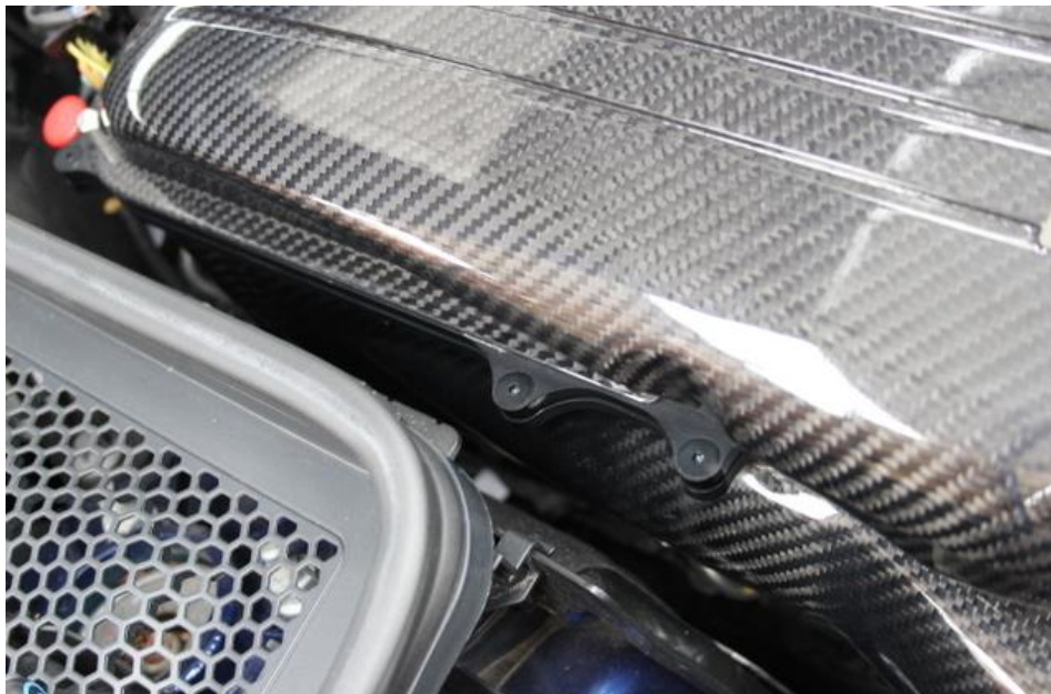
27. Secure the airbox with the supplied countersunk screws. Screws only need to be finger tight – do not put excess force on them.
