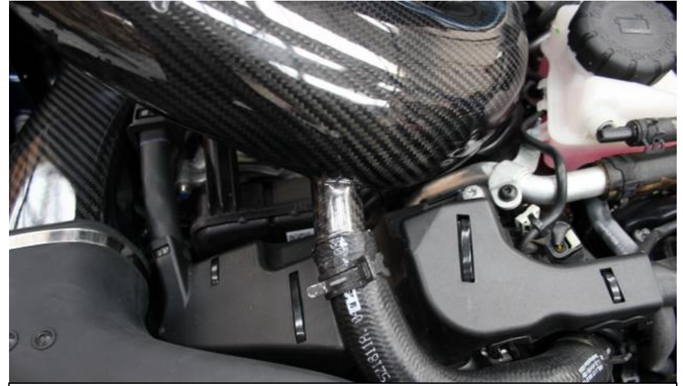
22. Take the Left side airbox lid and push the breather pipe into the front.
