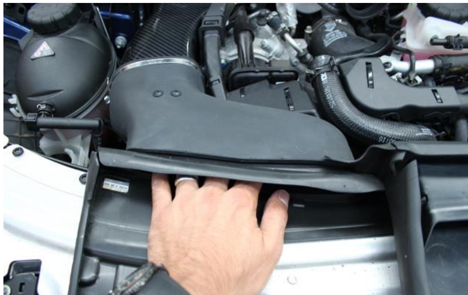
19. Push the rubber duct into place around the stock plastic duct trim.
