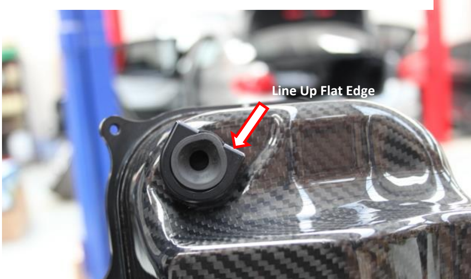
17. Rotate the mount holder on the Left side airbox so that the flat section lines up with the shroud from the previous step.
