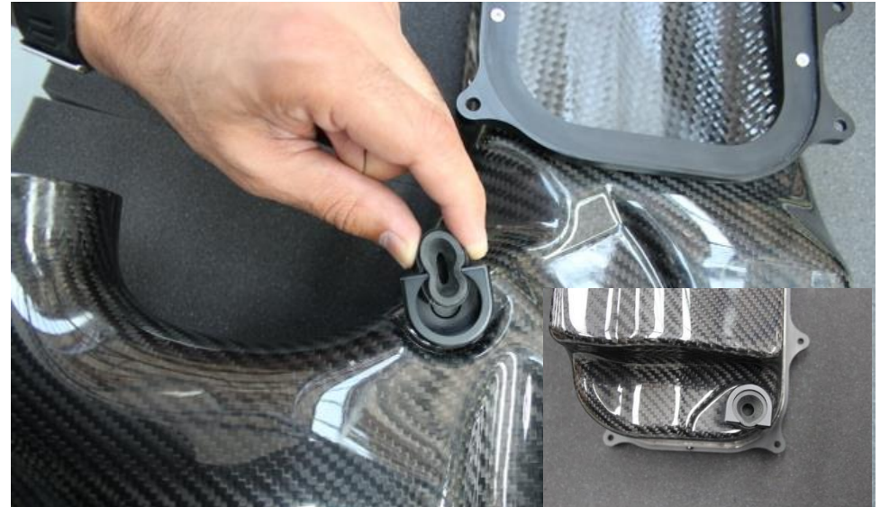
14. Push the rubber mounts into the mount holders on the carbon airboxes. There are 4 positions. One mount on each carbon piece. They can be pinched and pushed into the holders
