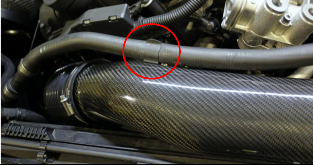
39. Push the stock rubber hose into the metal clip on the carbon tube.
