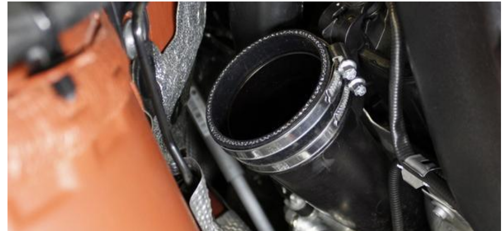
29. Taking the shorter 76mm coupler, push over the intake tube on the LEFT side of the engine. Make sure the coupler is pushed down fully and put two hose clamps around the coupler as shown. Tighten the LOWER clamp only.
