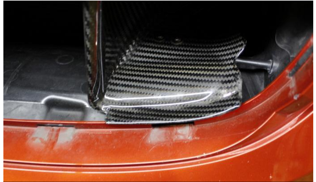
57. Lower lip should rest on the bumper grill panel. The scoop still needs to go further to the right to be in correct position. See next steps.
