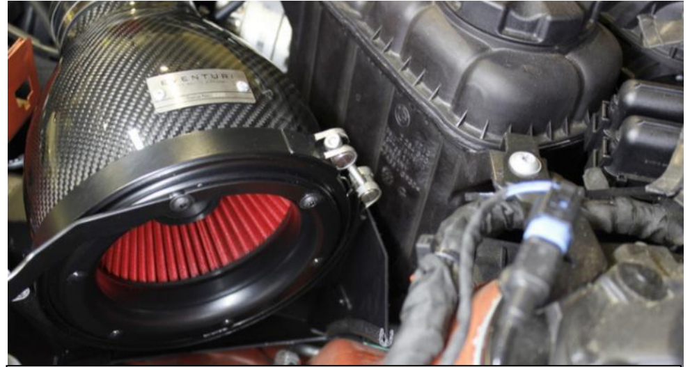
40. Place the mouth of the intake into the duct – rotate the Band Clamp to avoid the duct.
