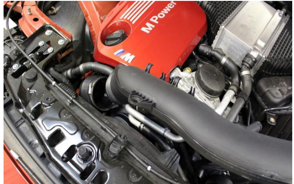
14. Loosen hose clamp and pull the tube out from the intake pipe.
