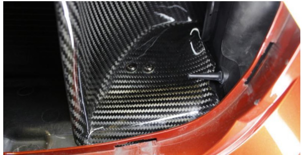
59. Pull the bumper area around the bottom of the scoop out to allow the lower lip of the scoop to go underneath as shown. The scoop should now locate as shown.
