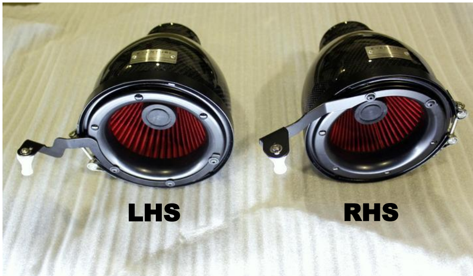
30. Identify the left and right side intakes. The left side has the mounting bracket secured around the bottom of the opening. The right side has it secure around the top as shown.
