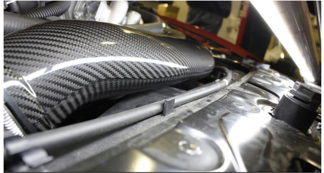
44. Rotate the carbon tube to allow a gap over the fan shroud. The hose clamps on either side of this tube should still be loose to allow rotation.
