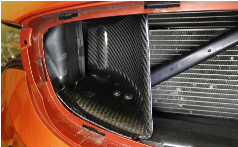
52. The scoop should be as shown with the lower lip against the top of the grill panel.
