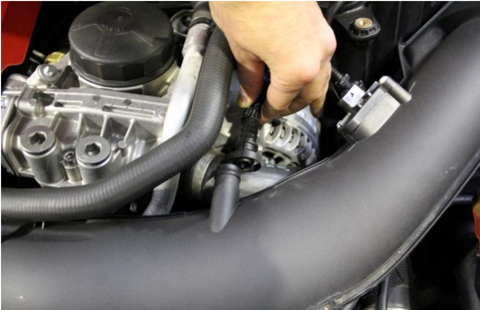
13. Remove Breather hose from tube. Pinch the sides of the plastic ring inwards and pull out.
