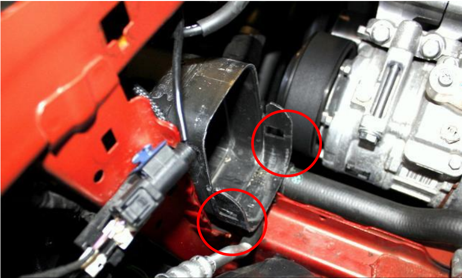
20. Starting from the right hand side (as you look at the engine) the stock duct opening has two holes which will be used to locate and secure the new duct.
