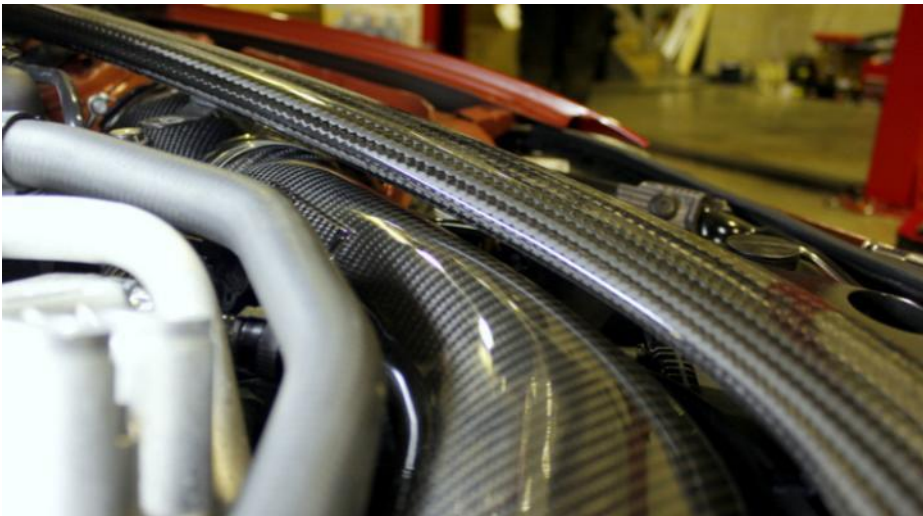
45. Place the strut brace into position to check for clearance above the carbon tube. Rotate tube if necessary. There should be a small gap between the tube and the strut brace and between the tube and fan shroud below. Remove strut brace.
