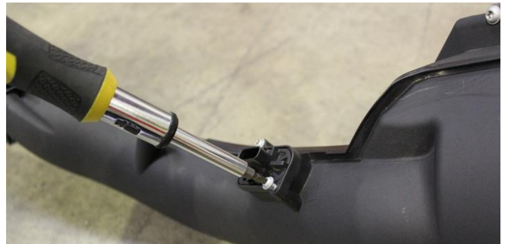
16. Using a Torx T20 – remove MAF sensors from both left and right side airboxes.
