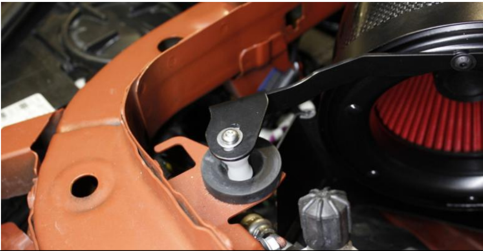
41. Locate the mounting boss over the stock rubber grommet. If required, rotate the mount and filter assembly in the housing. Band clamp should be loose enough to allow this – otherwise loosen to allow rotation.
