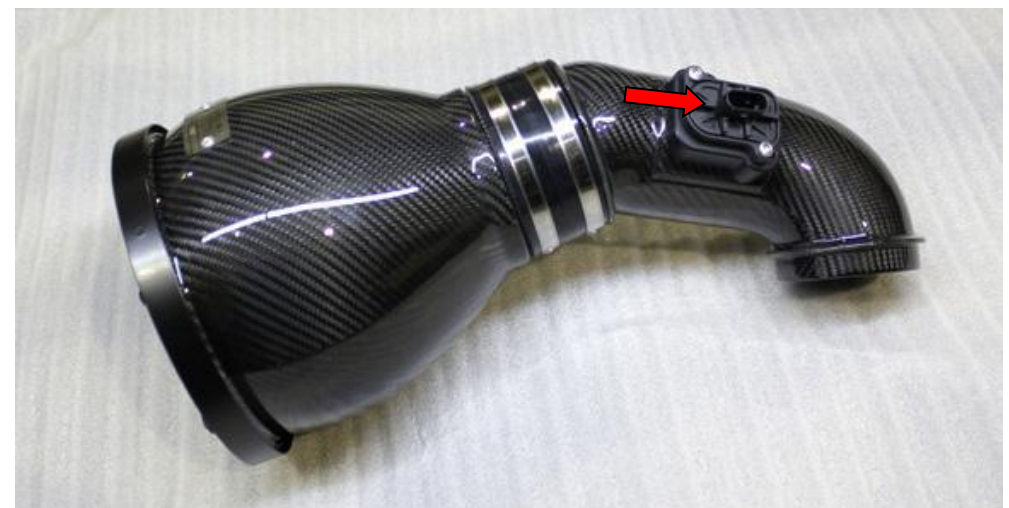
31. Assemble the LHS intake with the LHS tube (shorter tube) with the 80mm silicon coupler and 2 hose clamps. Orient the tube as shown here and in the next photo. When pushing the silicon coupler onto the intake – DO NOT PUSH ON THE FILTER ITSELF . Ensure airflow arrow on sensor is as shown.
