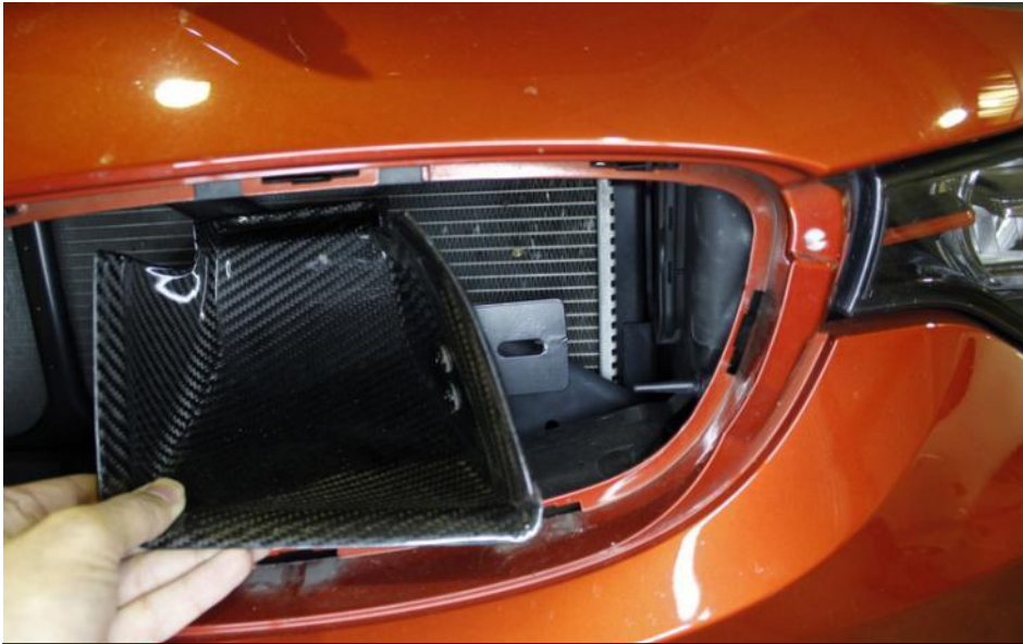
56. Take the RHS scoop and insert as shown with bracket facing the right side headlight. Once inside, rotate 90 degrees clockwise so the bracket faces down.
