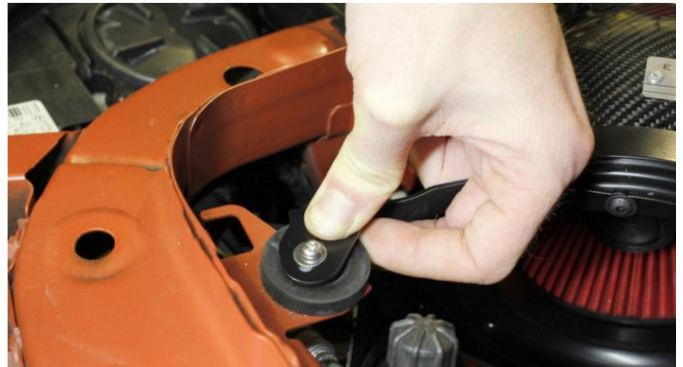
42. Push the mount all the way into the grommet.
