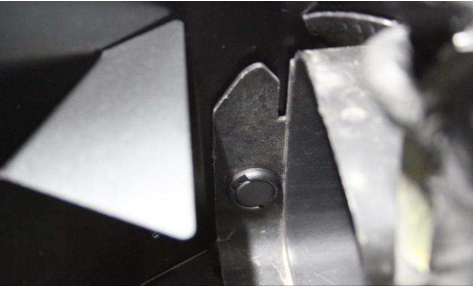
15. Push 1 rivet through the stock duct and secure the shield. The rivet will lock once the head is pushed in all the way.
