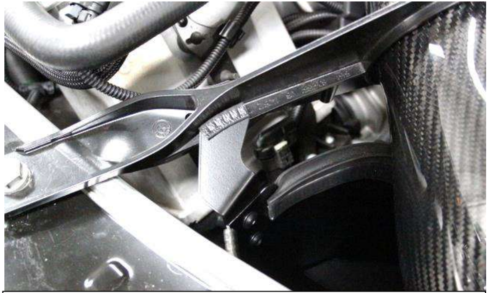
38. Repeat for the RHS bracket and secure again with the M5 screws and lock nuts.
