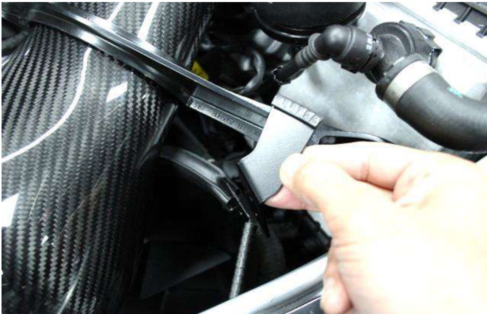
35. Take the LHS bracket and position it between the LHS shield and strut brace.
