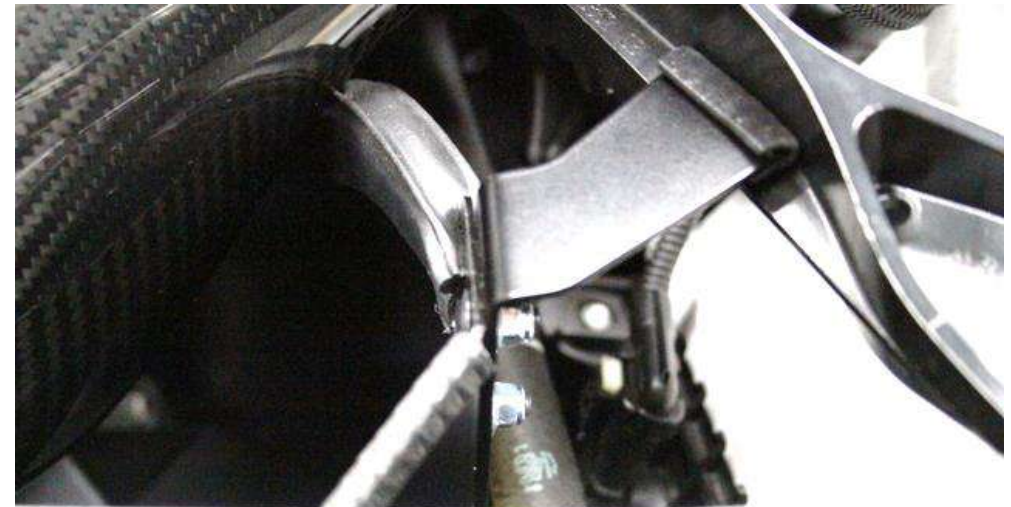
34. With both housings installed – we will now secure the shields. Take the supplied brackets and M5 screws with lock nuts. Identify the LHS and RHS.
