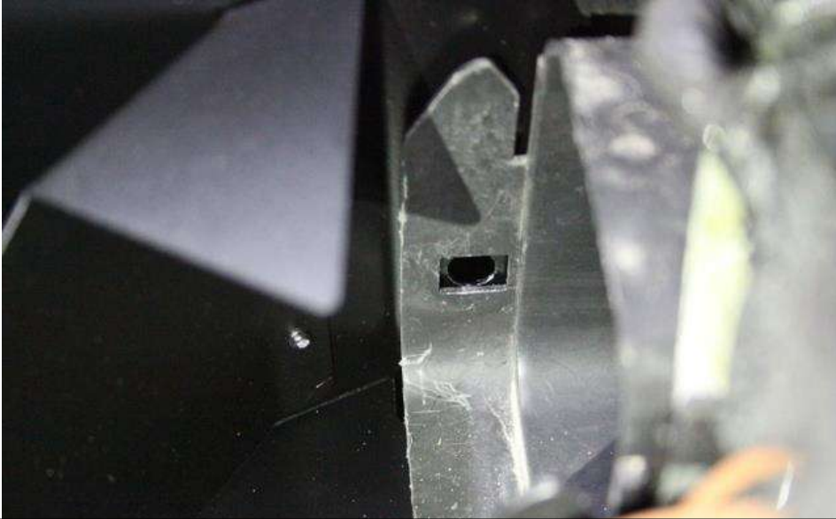
13. Line up the hole in the shield with the cutout in the stock duct outlet.
