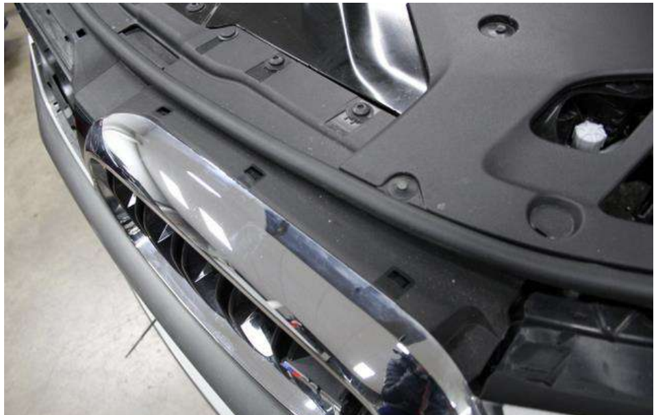
39. Remove the front grills – the tabs at the top can be pushed in while pulling the grills to remove them.
