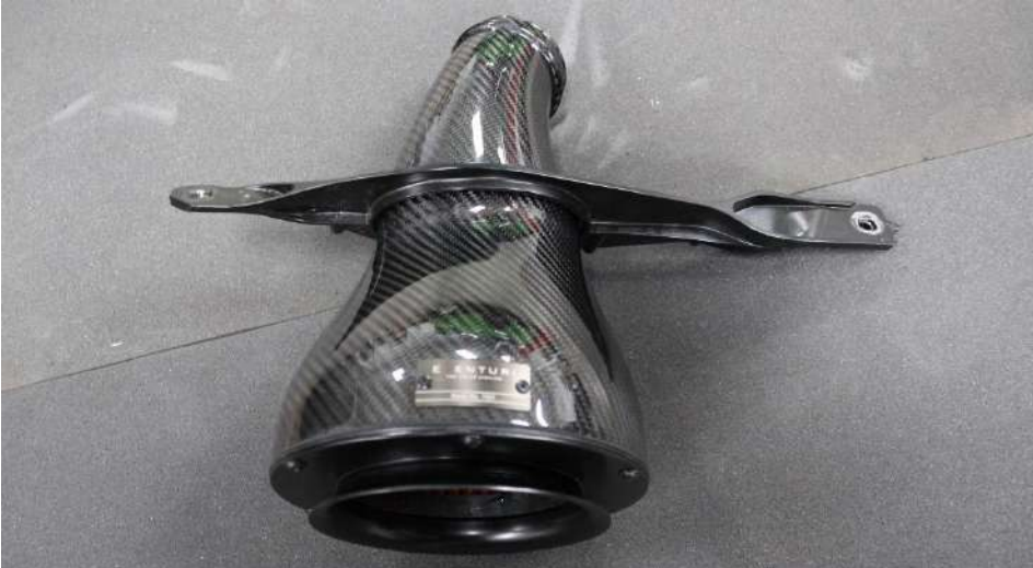
25. Take the LHS housing and feed it through the left strut brace. Notice the orientation of the brace against the housing.
