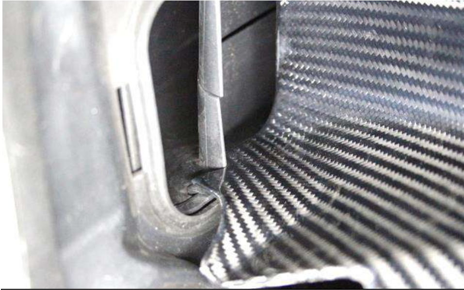
33. The start of the scoop should locate into the trim opening as shown.
