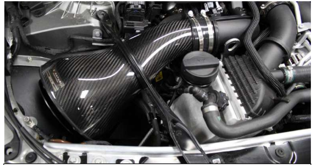
26. Lower is into place and push the housing into the silicon coupler. Do not tighten yet.
