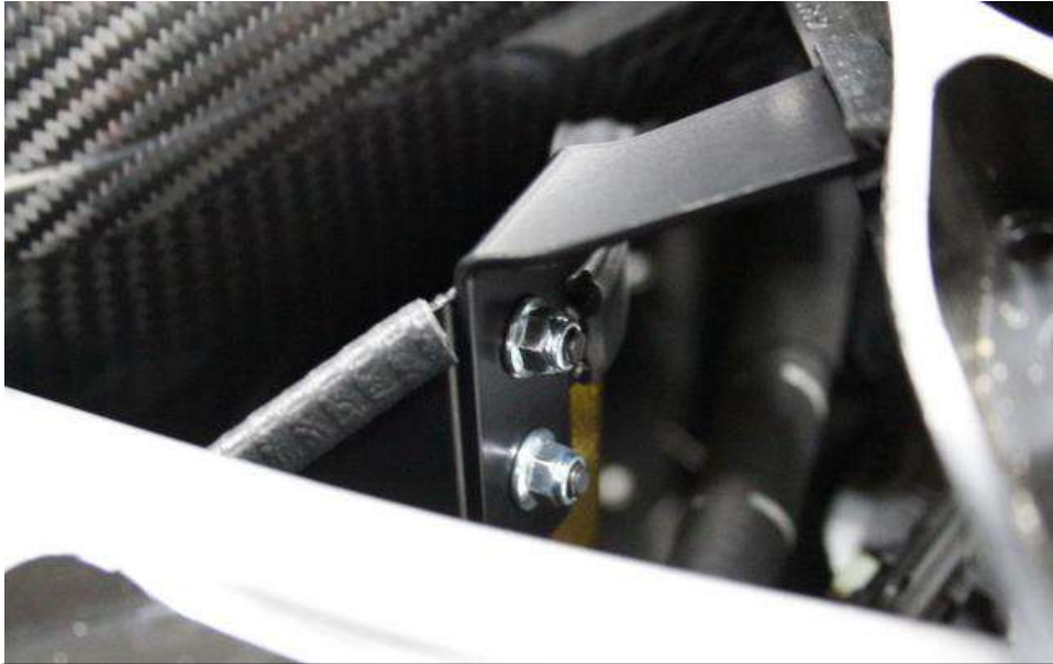
37. Another view of the secured LHS bracket.
