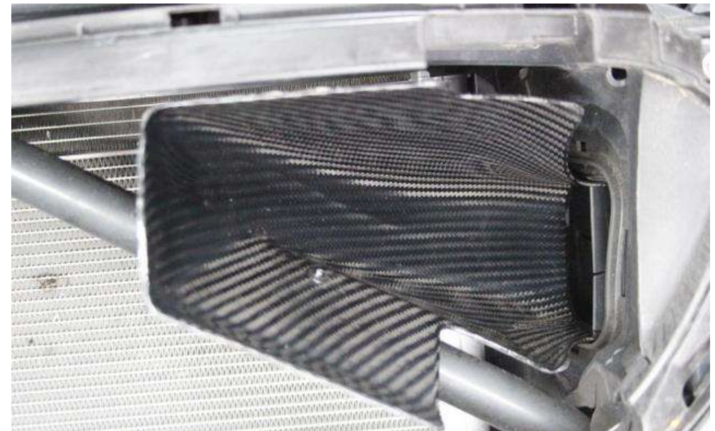
36. RHS Scoop installed.
