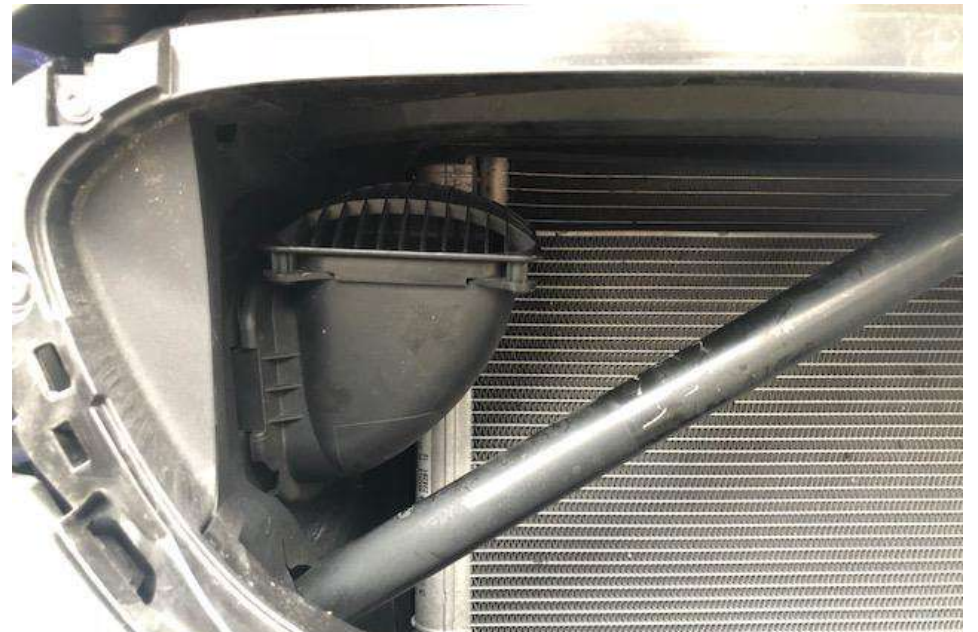
39. Remove the ducts behind the strut bar - these can be pulled out.
