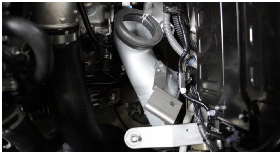
11. Start by pushing corner 1 over the RUBBER section of the cooler hoses and into the wheel arch area. The rubber hoses will be pushed down by the scoop to gain access.
