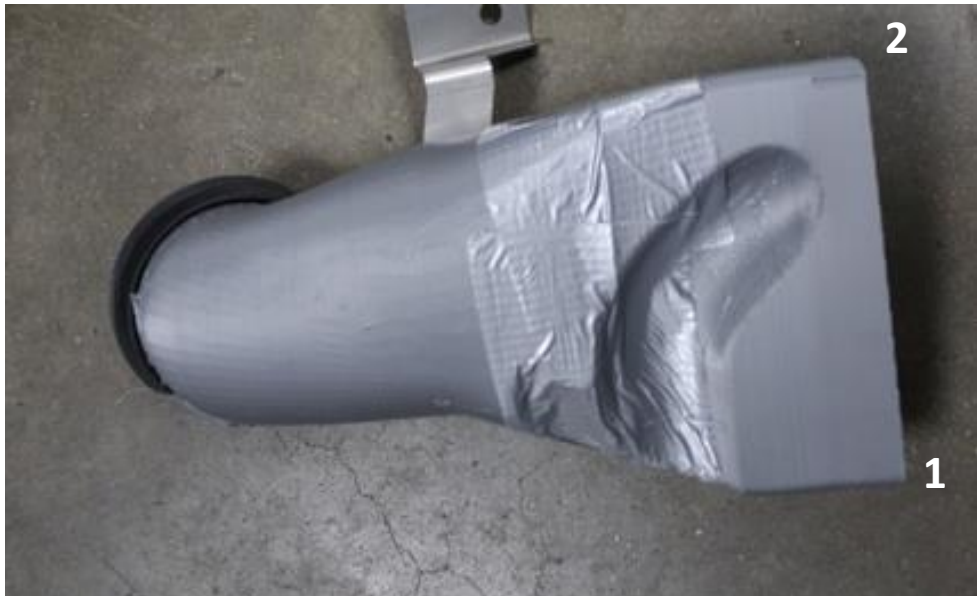
9. Take the scoop – notice the recess at the base – this is where the cooler hose will sit. Scoop shown here in grey for clarity. Notice the corners labelled 1 and 2. We will refer to these later.
