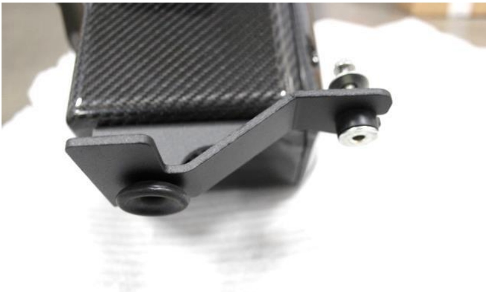
19. Insert the rubber grommet and 1 mounting bush into the front lower bracket of the airbox. Some lubrication around the outside of the rubber grommet will help.
