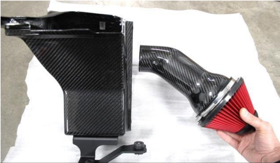
31. Push the carbon tube through the airbox as shown.
