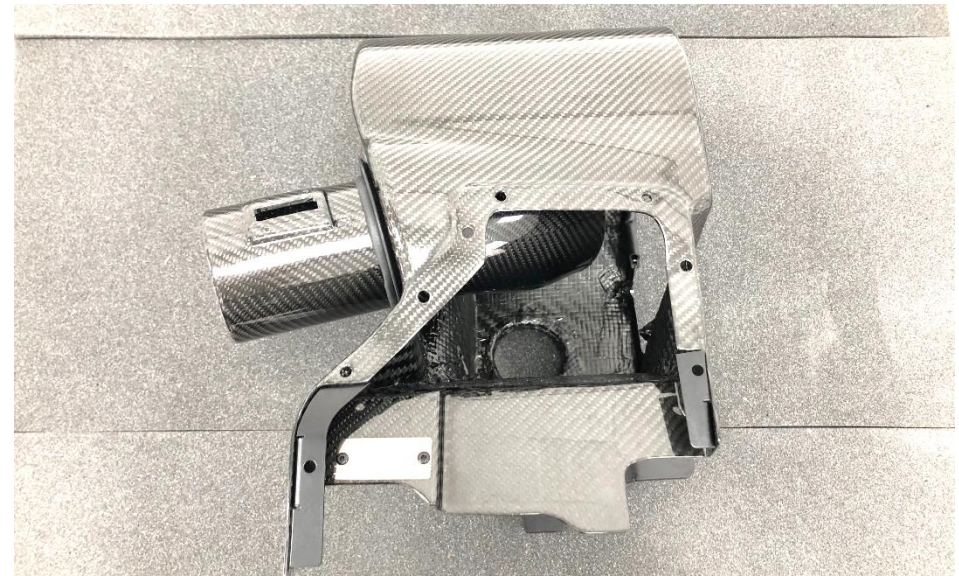
24. Push the carbon tube through the airbox as shown. (Filter not shown here)
