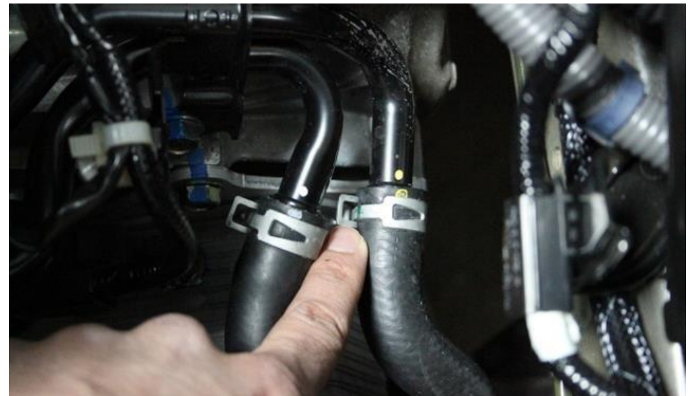
8. Rotate the clips on the oil cooler hoses so that the tall ends are on the side. We need this for clearance with the scoop.
