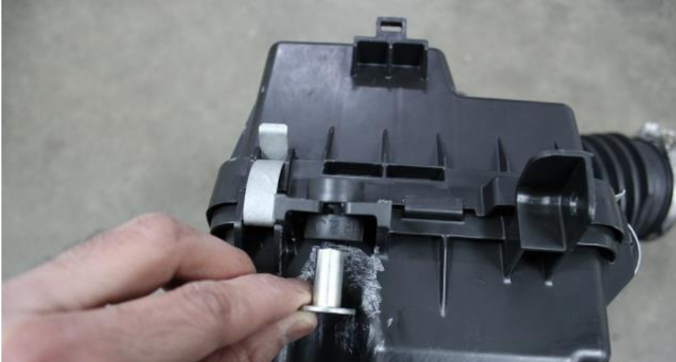
17. Rubber mounts can be removed by sliding out the metal bush and then squeezing out the rubber.
