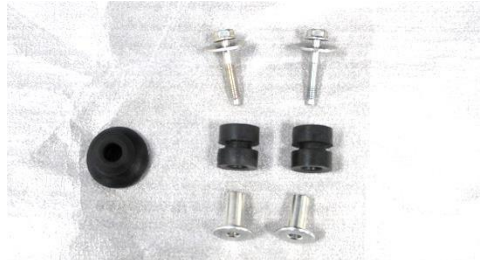
18. Here are the 2 rubber mounts with bushes and bolts and the rubber grommet removed from the airbox.
