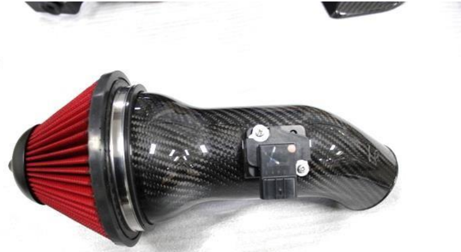
30. If your carbon tube already has the pre-installed Metal MAF sensor mount then you can simply install the MAF sensor as shown and secure the filter to the tube.
