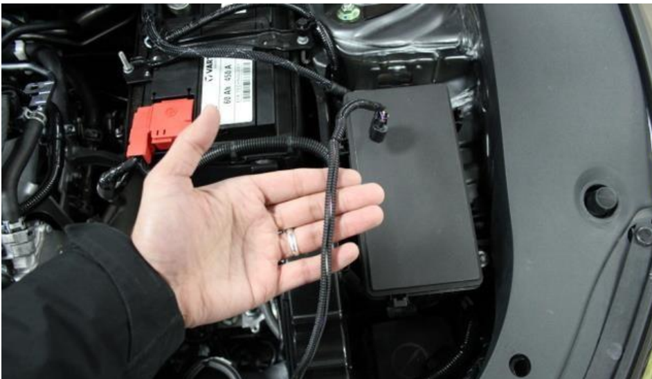
15. Insert the exposed MAF sensor plug wiring into the supplied cable shroud.
