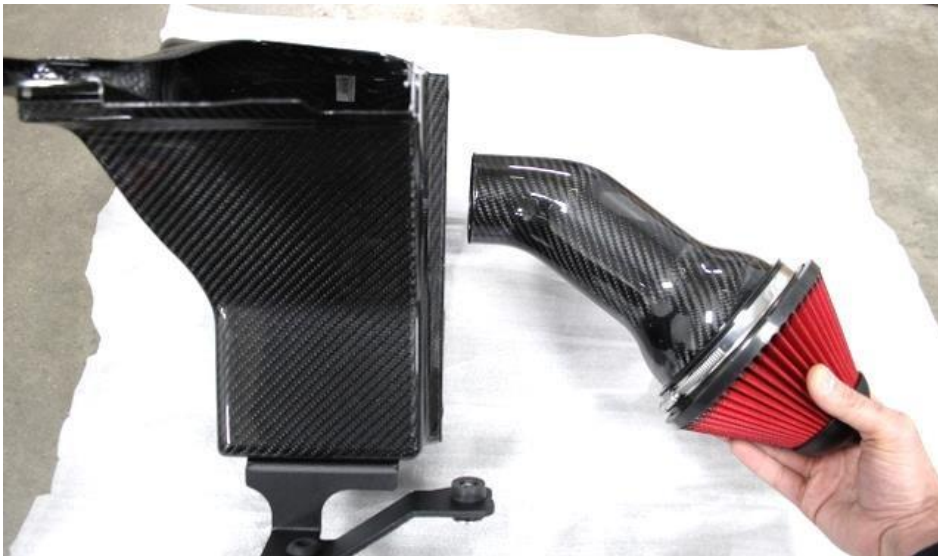
23. Install the filter onto the tube and secure with the clamp – then push the tube through the airbox.
