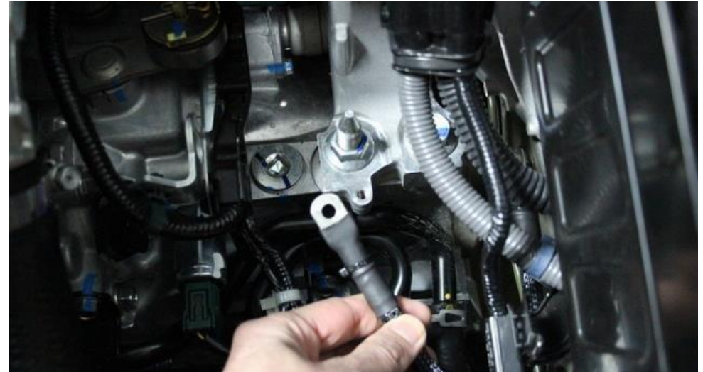
6. Remove the bolt holding the strap in place.
