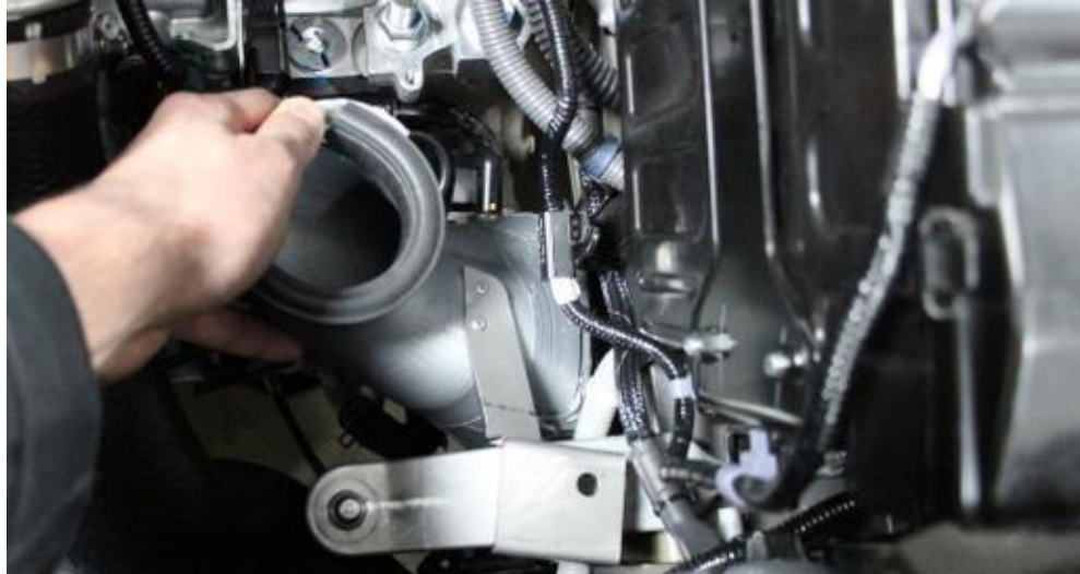
12. Once the corner is pushed into place, push the scoop upwards and rotate the scoop to push corner 2 into place. The recess shown in step 9 will go over the oil hose and the bracket should line up with the OEM metal mount location.
