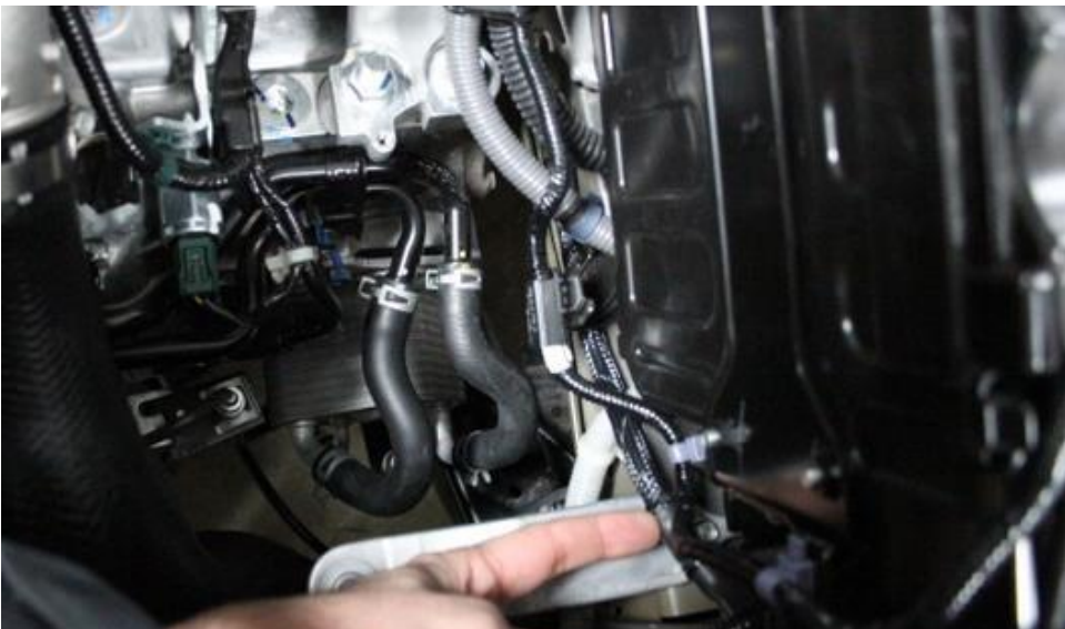
7. Push the strap out of the way to get clearance for the scoop installation.
