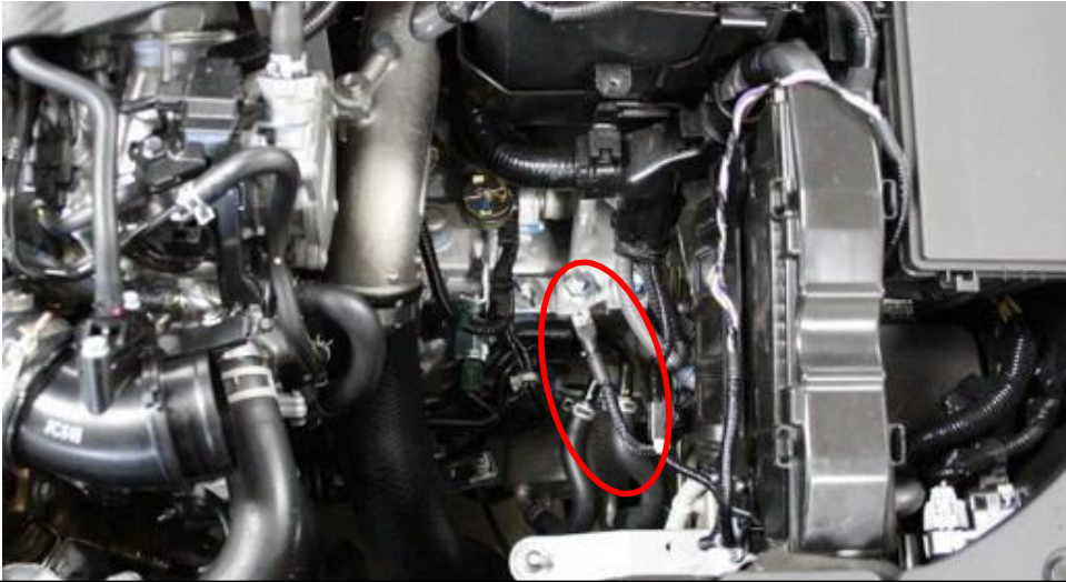
5. Locate the earth strap as shown.
