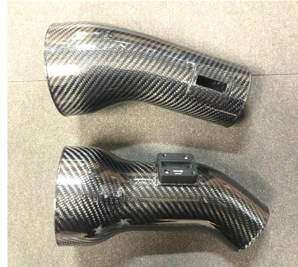
22. If your carbon tube looks like the top one and does NOT have a pre-installed metal MAF sensor mount then proceed to the next step. If your tube looks like the bottom one and already has the MAF Sensor mount installed proceed to step 30.
