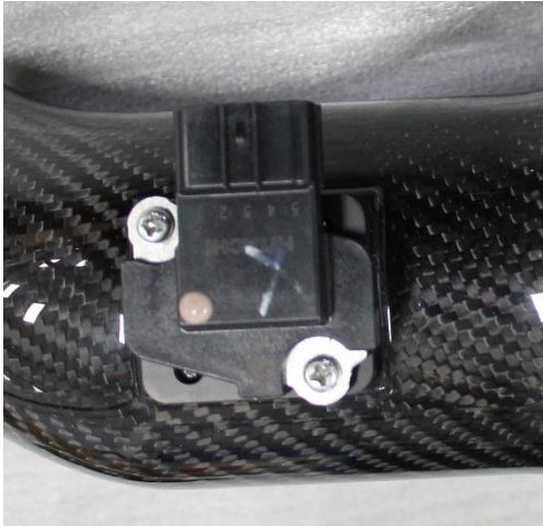
29. Install the MAF sensor using the other 2 screws from step 25. Now proceed to step 33.
