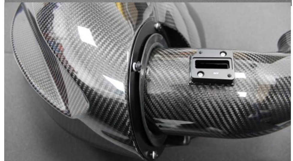
16. Insert the filter into the airbox and line up the holes on the sealing plate. Secure with the supplied M5 screws and lock washers.
