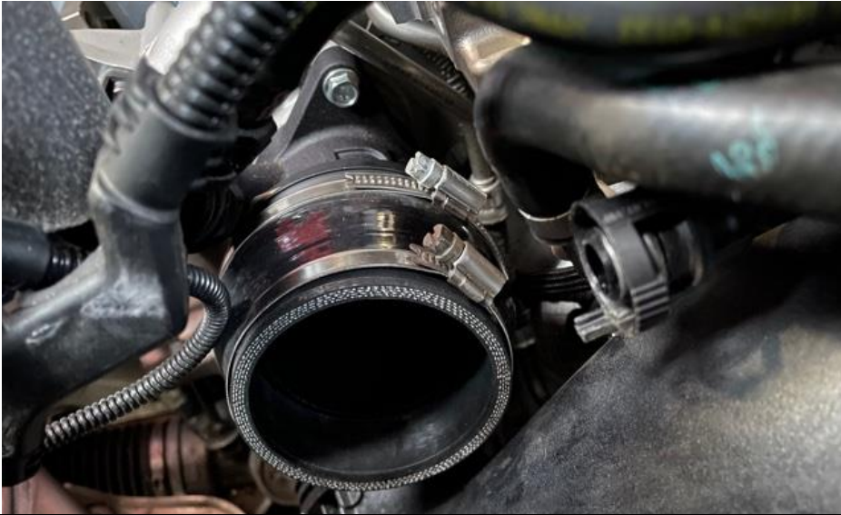
13. Install the flange assembly onto the turbo inlet – it will click into place.
