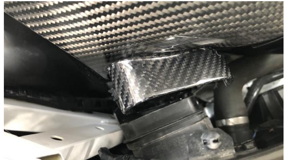
24. Bring it down at a slight angle with the front duct to locate the mounts and the secondary scoop as above.
