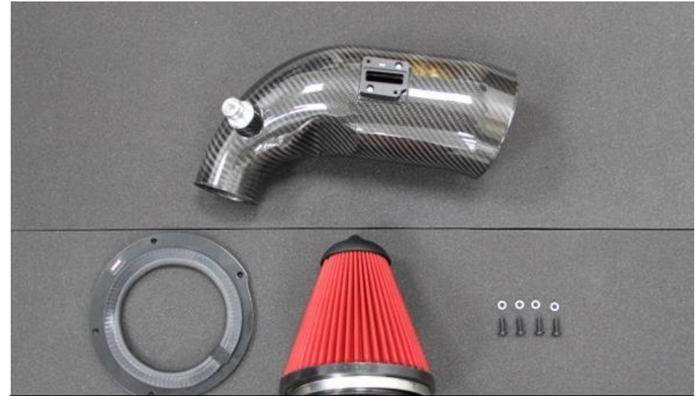
14. Take the inlet tube, filter, sealing plate and the M5 screws with lock washers.
