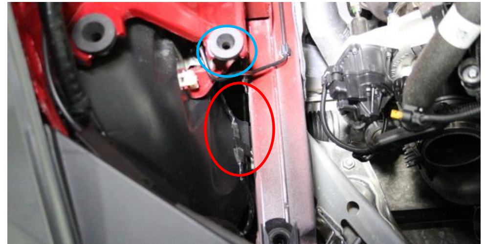
20. Gap in the wheel arch area and rubber mount.
