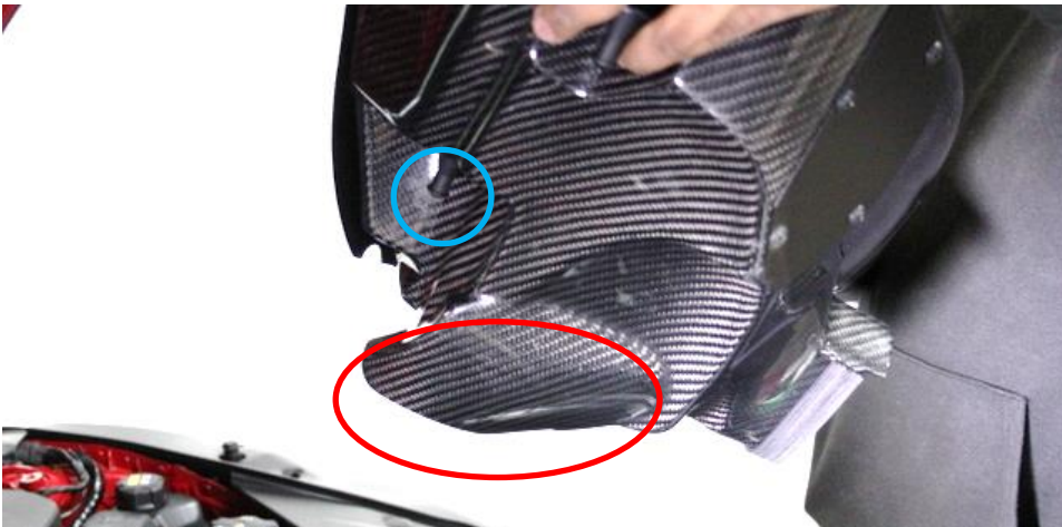
19. Carefully lower the airbox into the engine bay. Note that the secondary scoop circled above goes into the gap shown in the next photo. Also the mount circled blue should sit in the rubber mount shown in next photo.
