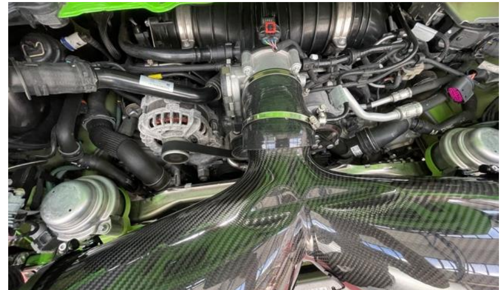
16. Push the intake into the silicon as you rotate it into the engine bay.
