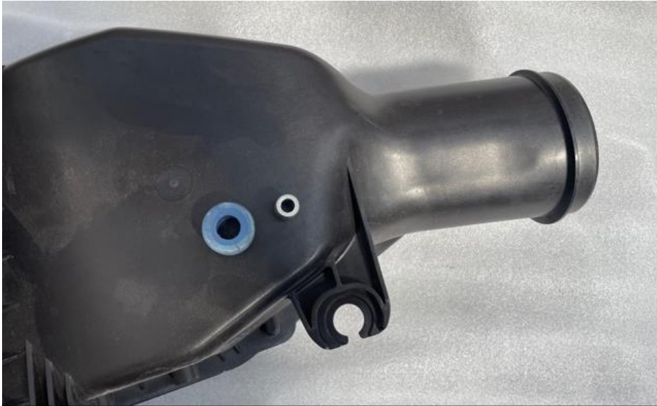
13. Remove the mounting bushes from each side of the airbox.
