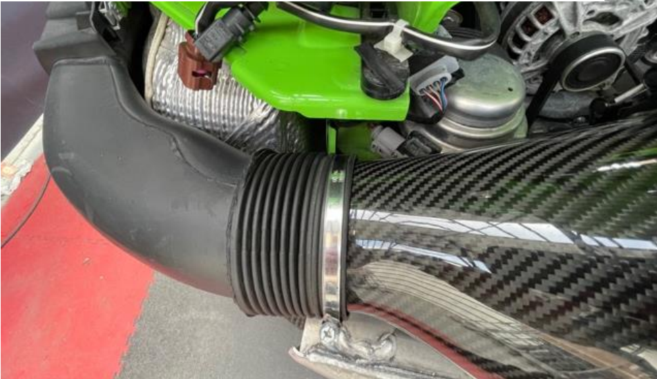
17. Here is the Right side in place. Notice the tab on the base is again in front of the tab on the chassis and the rear panel on the shield is under the stock duct.
