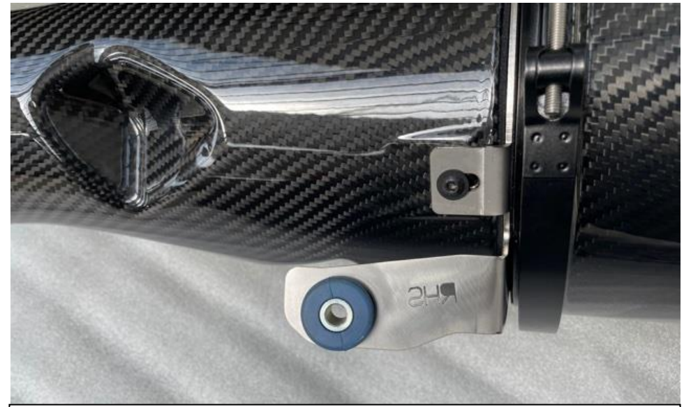
14. Insert the bushes into the new brackets of the intake.
