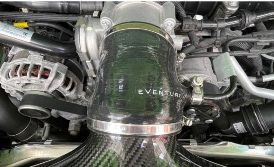
19. Tighten the clamp around the intake – make sure the intake is fully inside the silicon. Don't overtighten – the carbon can be damaged if overtightened.
