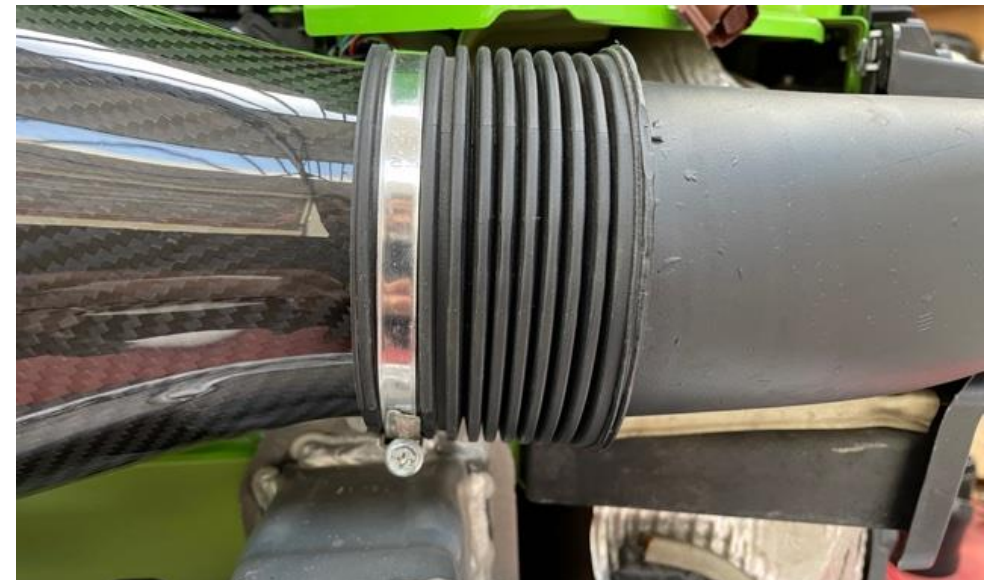
20. Secure the clamps around each duct. Don't overtighten.
