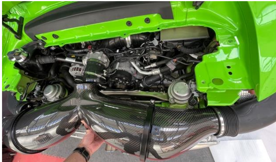
15. Now take the intake and push the right side into the right inlet duct – (right duct is on your right as you look at the engine from behind the car)
