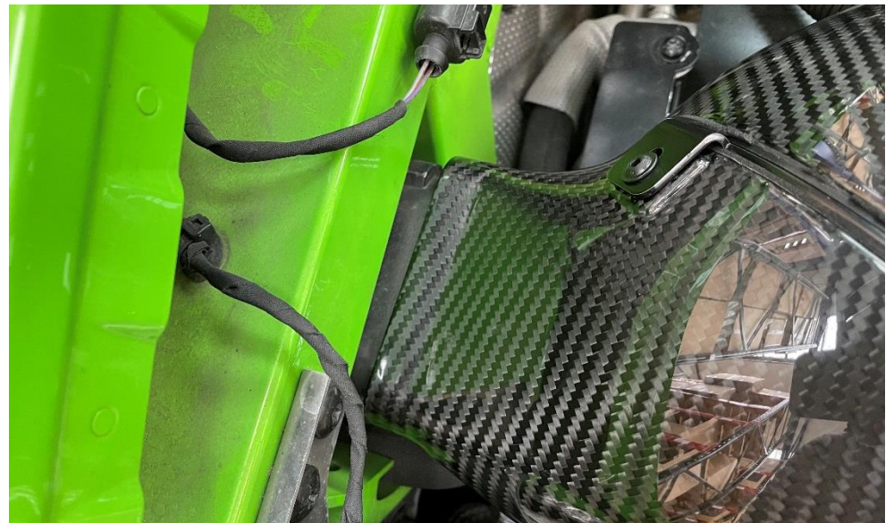
25. The intake should go over the stock air feed.
