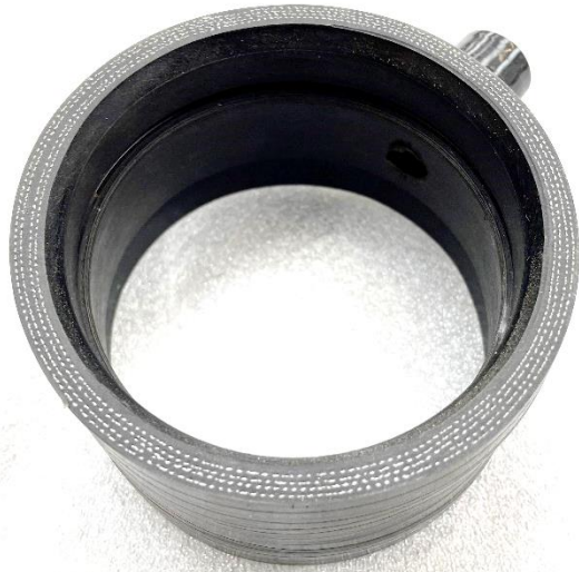
22. Take the silicon couplers and install them onto the throttle bodies.
