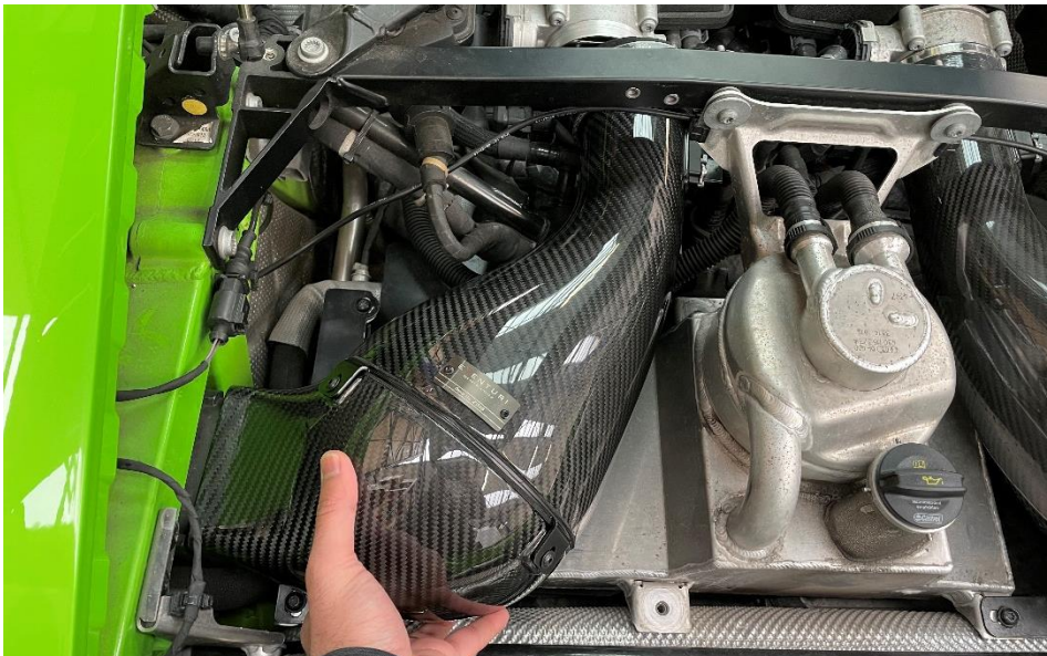
24. Position the left side intake into the silicon and push into the stock air feed.
