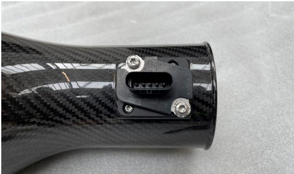
15. Insert the sensors into the Eventuri intake tubes. Make sure the orientation is correct. Use the supplied Torx screws to secure them. DO NOT USE THE STOCK SCREWS.
