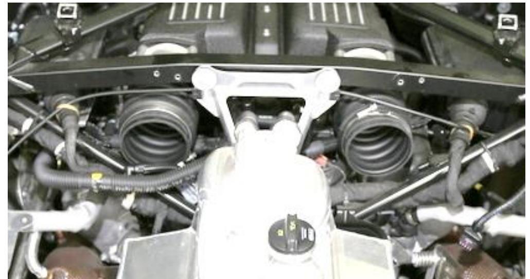
16. Remove both of the flexible rubber hoses from the throttle bodies.
