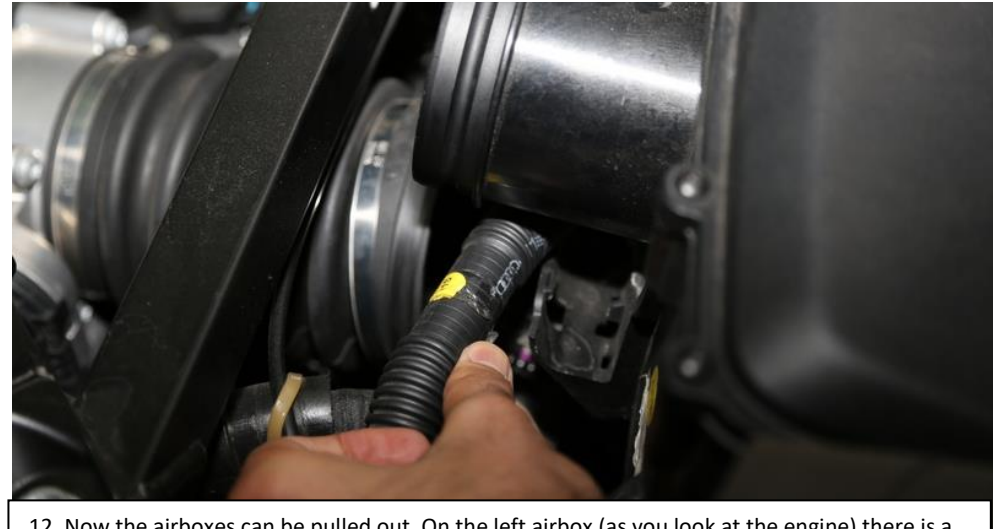
12. Now the airboxes can be pulled out. On the left airbox (as you look at the engine) there is a hose which needs to be removed from the airbox as shown. Remove both airboxes completely. On the Audi R8 you will need to disconnect the vacuum line to the secondary flaps on the airbox. We will plug this later.
