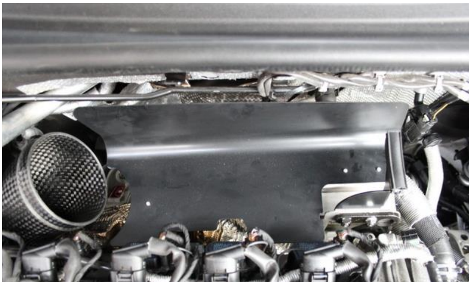
18. Lower the shield at the back of the engine as shown. (Optional Carbon turbo inlet shown).
