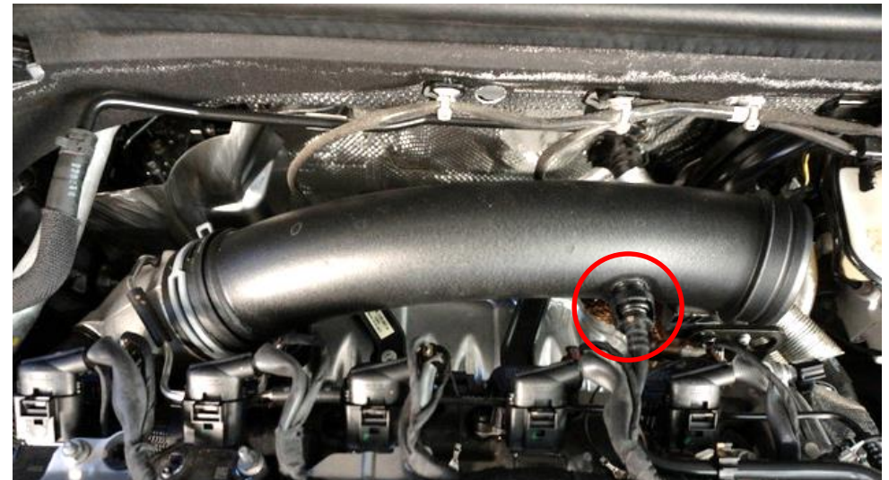
5. Remove the spring clamp holding the turbo tube to the rubber joiner and also the breather connector circled in red.
