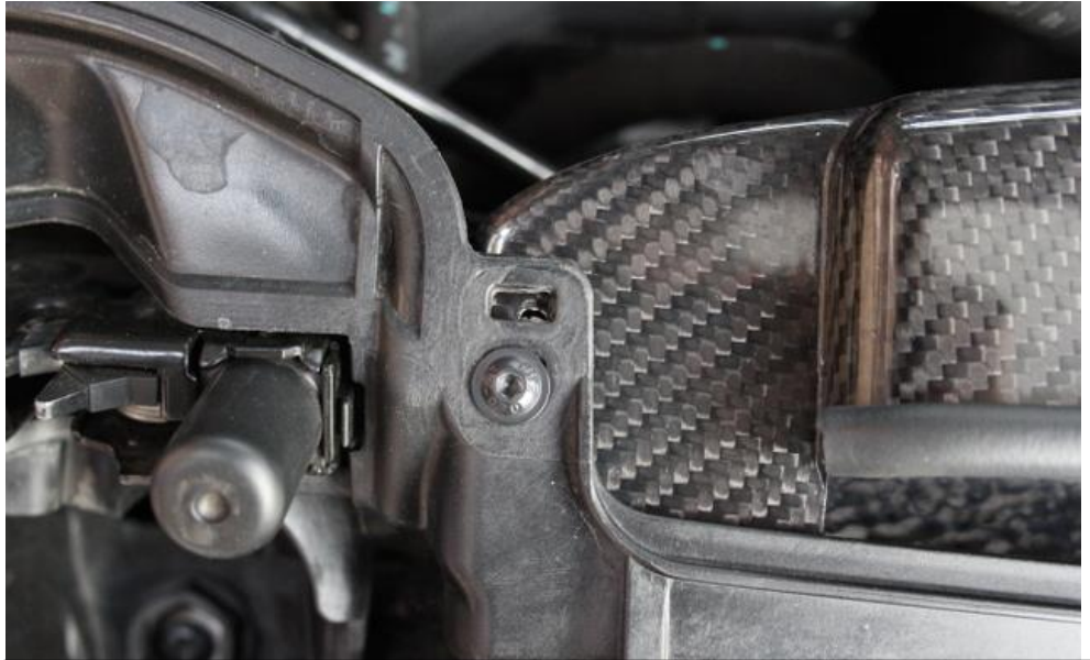
41. Line up the hole on the panel with the correct hole on the duct as shown in previous step. For RS3 Secure with a supplied M5 Screw. For RSQ3 secure with the original stock screws.
