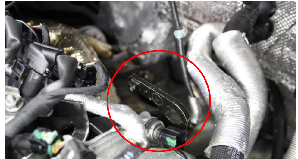
17. The shield and tub bracket are mounted together to the same location at the back of the engine where the OEM tube was fixed (Step 5). If there is a cable attached by a clip to this bracket – remove also.
