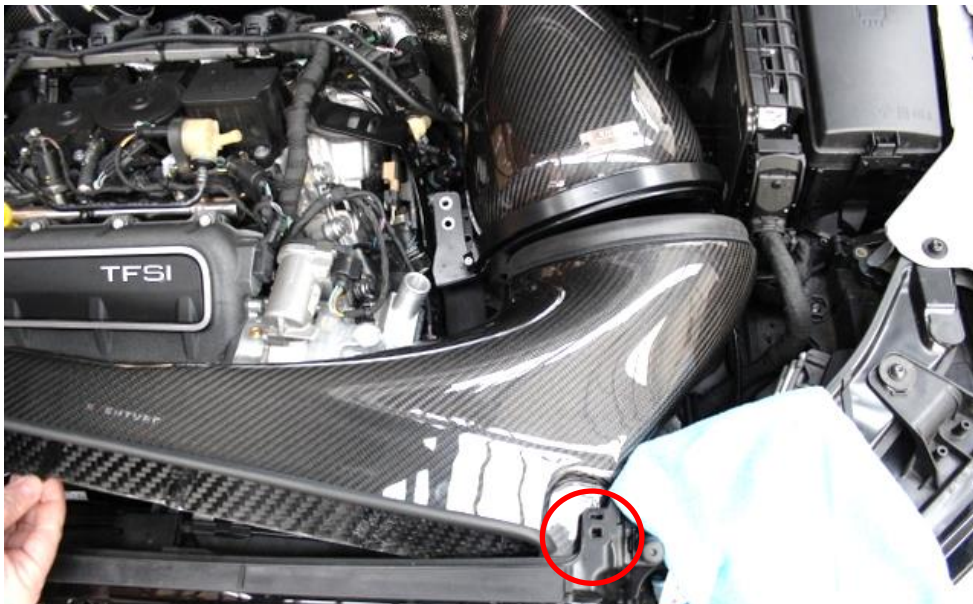
38. Now rotate the duct so the rear corner goes into the mounting location circled.
