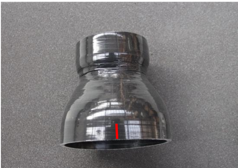
22. Mark the high point with a pen.
