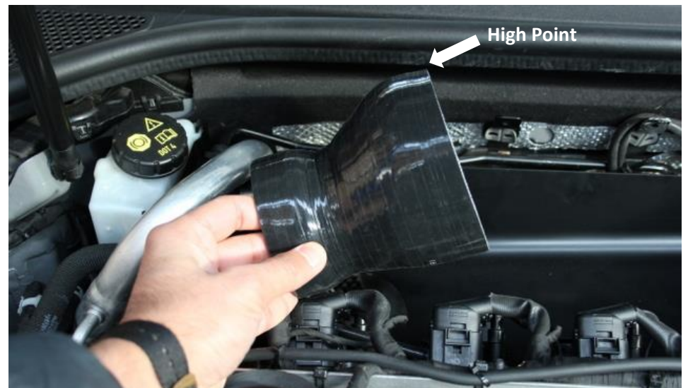
23. Place the reducer onto the stock turbo inlet tube with the appropriate hose clamps and the high point facing upwards as shown.
