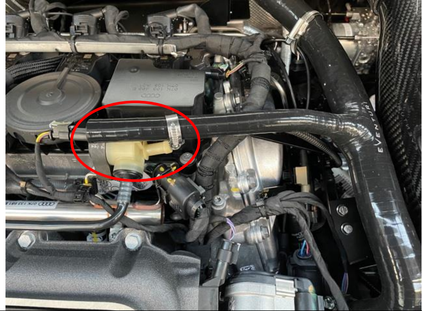
47. Install the breather hose as shown - you may need to trim the hose as shown.
