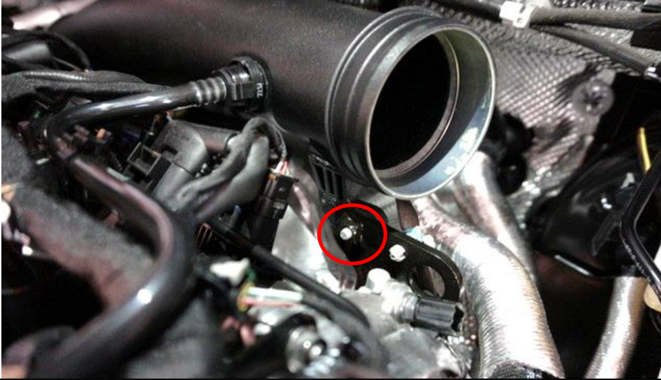
4. Remove the screw securing the Turbo Tube.
