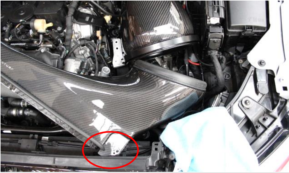
36. Carefully angle the duct down as shown. The rubber seal will touch the filter housing and the back edge should go inside the slam panel as circled. See next photo for another angle.
