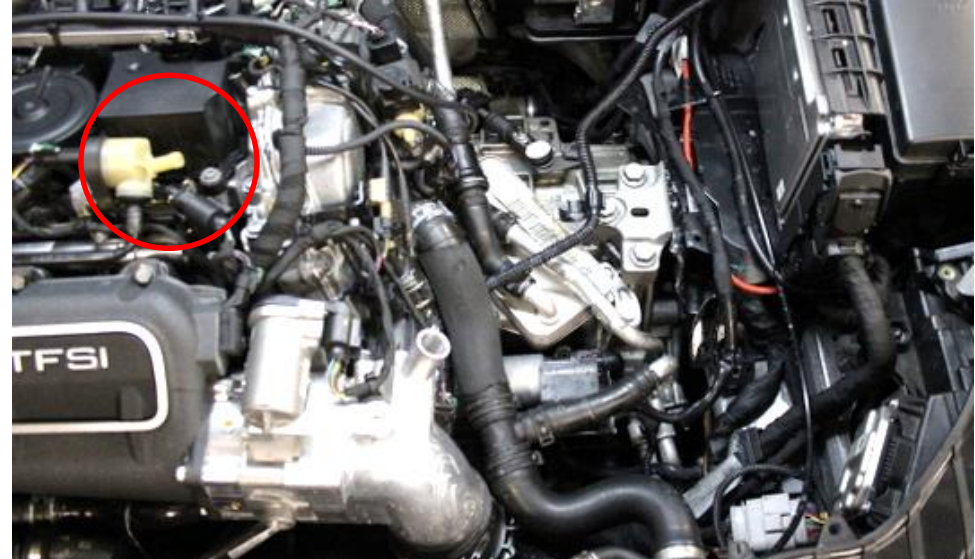
15. Remove the breather tube from the yellow breather module.
