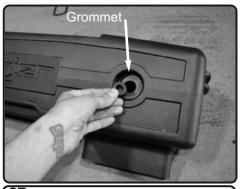
**27.** Install the grommet to the hole on the air box.
