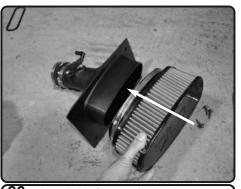
**26.** Install the filter to the intake plenum, secure and tighten using 8mm nut driver.
