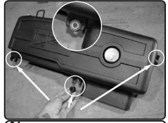
**31.** Now install the factory grommets with crush washer removed from the OEM air box (step 20)
