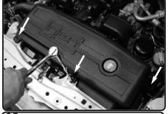
**35.** Secure and tighten all the screws using 10mm socket or wrench.
