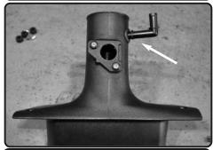
**22.** Install the provided grommet to the hole on intake plenum. Install the 90 degree plastic elbow long side first to the grommet and secure.
