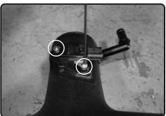
**24.** Secure the MAF sensor using provided M4 screws and tighten 2.5mm allen key.
