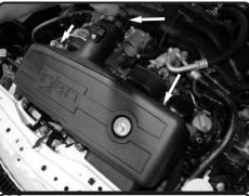
**32.** Push hump hose foward allowing for hose to slide back. Install the injen evolution intake assembly into vehicle.
