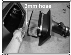
**29.** Now attach the 3mm hose to the fitting on the filter.
