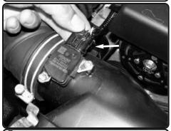
**5.** Disconnect MAF sensor harness and pull line away from air box.
