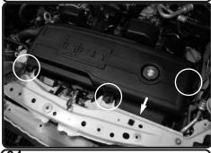
**34.** Make sure the injen box and the scoop are attached. Make sure the gasket is sandwiched between. Now secure the air box using the factory screws from step 7.
