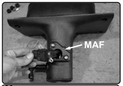
**23.** Remove the MAF sensor from the stock air box, install the MAF sensor into the new intake plenum.
