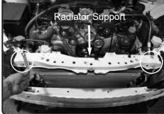
**12.** Loosen the 4 bolts on top of radiator support using 12mm socket or wrench. This will be for installation of Ram Scoop.
