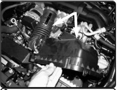
**6.** Un-clip the upper part of the air box, remove the upper assembly including the intake tube from the vehicle.
