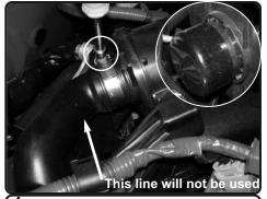
**4.** Loosen the clamp on the Sound Tube resonator. Loosen the clamp on the intake tube and remove the sound tube. This will no longer be used on the new Injen intake system. Use provided Vinyl cap and cap off sound tube.
