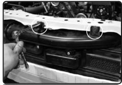
**10.** Remove the air box resonator by loosening the 2 bolts.
