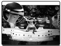
**13.** Locate the 2 remaining bolts on bottom of the radiator support in front of exhaust manifold loosen and remove.
