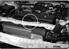
**38.** Secure the MAF sensor using provided M4 screws and tighten 2.5mm allen key.
