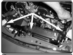
**7.** Loosen the 3 screws holding in the bottom half of the air box using 10mm socket and ratchet. Now lift up and remove the lower intake assembly from vehicle. Save for later install.
