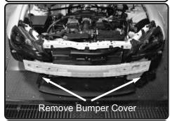
**9.** Carefully remove bumper cover. Remove the push-clips and 10mm screws on top and bottom and side and remove.
