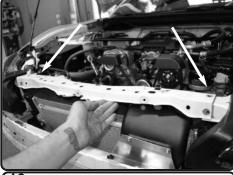
**19.** RE-install the radiator support and secure. Re-install the bolts and tighten.
