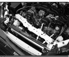
**14.** Push back radiator support allowing for the install of the injen ram scoop.
