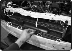
**11.** Remove the plastic splash guard from the front of vehicle, disconnect the push clips and remove.
