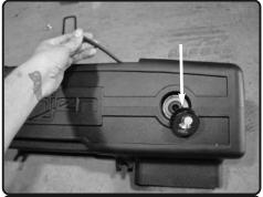
**28.** Attach the 3mm hose to the filter minder. Now install the hose through the grommet, secure the filter minder and make sure seats in grommet properly
