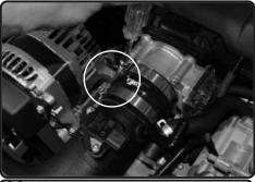
**36.** Now adjust the hump hose, secure and tighten the clamps using 8mm nut driver.
