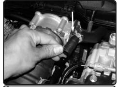
**3.** With pliers, pull back the crank case line from the intake fitting.
