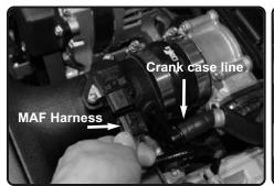
**37.** Secure and tighten all the screws using 10mm socket or wrench.
