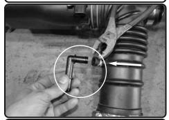
**21.** Remove the plastic 90 degree crank case elbow from stock intake tube.
