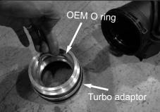
**10.** Now install the OEM O ring into the turbo adaptor.
