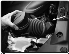
Remove the intake tube out of vehicle.
