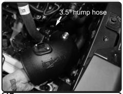
**17.** Install the intake into the tube and secure to the hose. Tighten clamp using 8mm nut driver.
