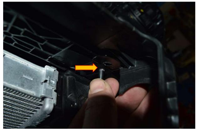
23. Drop in the FMCCRAD12 into the position where the OE radiator used to be and re-connect the upper and lower couplers.
