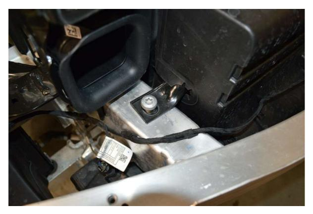
17. Disconnect the air temperature sensor, then remove the plastic cowling.
