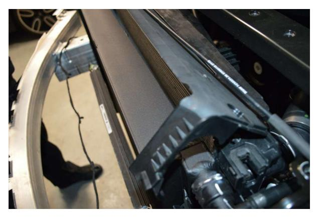
24. Mount the PAS cooler to the FMCCRAD12 to the machined bosses, use the two machined plates and four M5 fasteners to attach the PAS cooler in firmly place.
