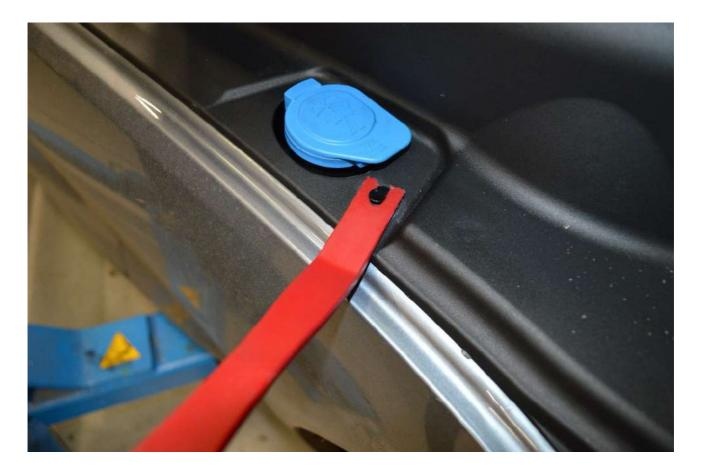
2. Remove the bonnet seal at the front of the engine bay, this just pulls off. With the seal removed you will see six M8 fasteners holding the top of the bumper in place. Use a 13mm socket and ratchet to remove them.
