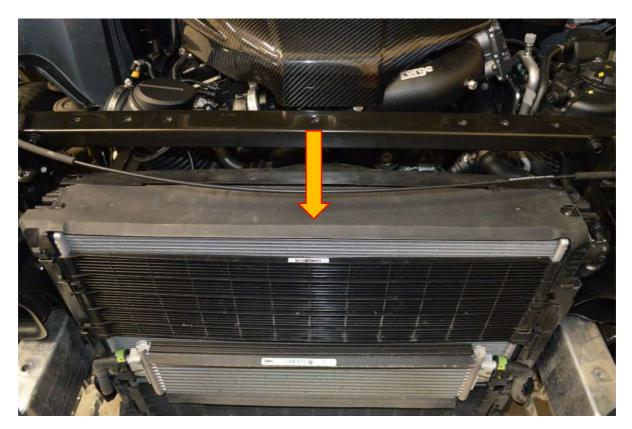
**19**. Remove upper and lower radiator grills from the OE charge cooler radiator, slide the grill upward while pulling the retaining clip. THESE GRILLS DO NOT GET RE-FITTED.
