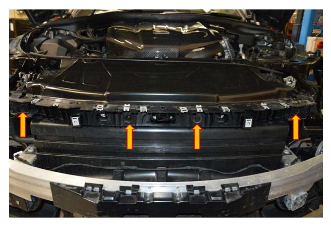
**11**. Remove the metal slam panel, which is held in place with thirteen 13mm fasteners. Like previous steps use the relevant socket and ratchet to remove them.
