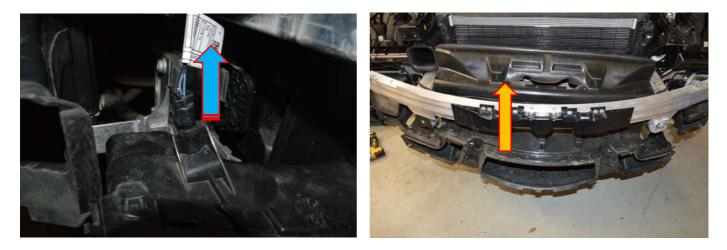
**18**. Remove the radiator top plate, there are two T30 Torx fasteners holding it in place, remove both fasteners and un-clip the top plate.
