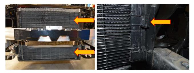
20. Remove the PAS cooler from its brackets BUT DO NOT DISCONNECT FROM ITS HOSES.
