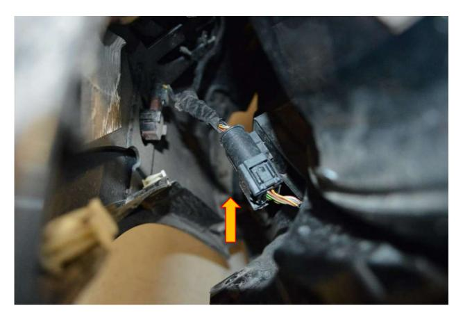
6. Unclip the loom to the pedestrian crash protection system, there is a plug on both sides that needs to be unclipped. Now remove the foam cover from the crash bar.
