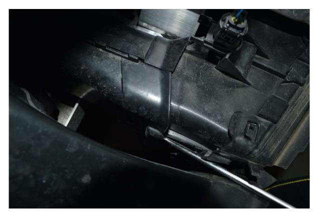
14. Remove the lower crash bar. The crash bar is held in place with four 13mm fasteners and six E10 fasteners. Use the appropriate socket and ratchet to remove all these fasteners.
