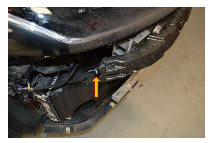
7. Remove the four T30 Torx fasteners which attach the bumper reinforcement.
