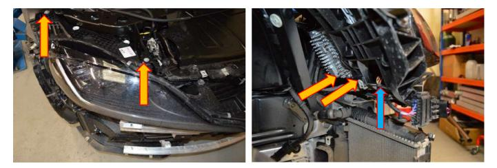
**10**. Remove the plastic slam panel, there are four M10 fasteners attaching this to the vehicle, use the relevant socket and ratchet to remove them.
