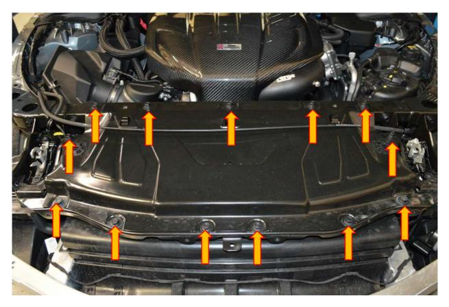
12. There is a slam panel locating bar which needs removing, it is held in place with four 13mm, two T50 and two T30 fasteners.
