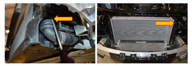
22. The tabs that hold the PAS cooler need to be cut down, use a junior hack saw and make your cut as shown in the picture below. You will need to do this on both sides. There is also a locating pin which needs to snap or be cut off at the top of the radiator.
