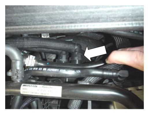
9. Using a sharp knife, cut the crankcase breather hose as close to the end of the spout as possible.
