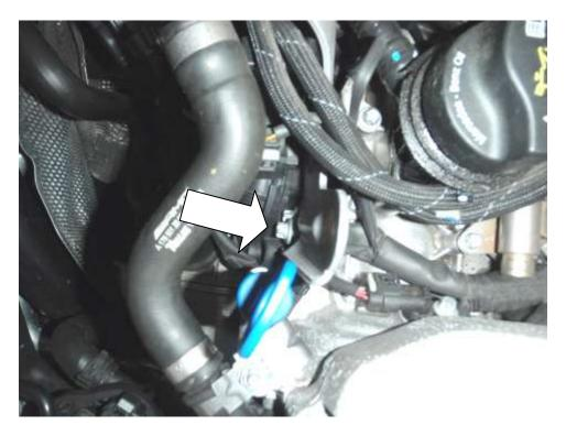
4. Ensure that the drain tap at the bottom of the catch can is in the closed position. Place the Forge Catch can in the cavity at the back of the engine.
