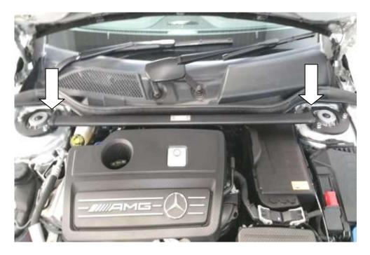
2. Pull the engine cover up firmly to remove it.
