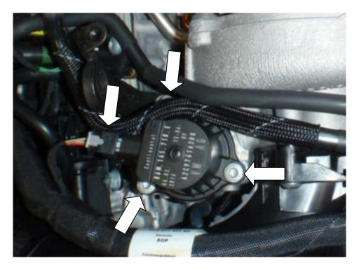
4. Ensure that the O-rings on the bottom face of the Forge dump valve are correctly installed and secure the valve in position using the 3x OEM bolts.
