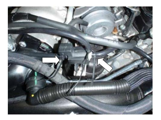
11. Using the custom wiring loom provided connect the OEM dump valve wiring to the solenoid.
