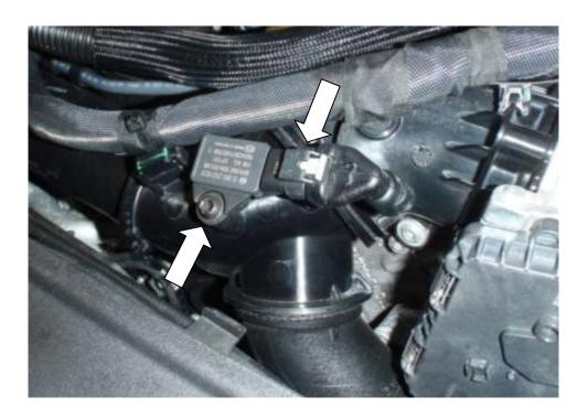
6. Install the boost take-off supplied into the hardpipe and reinstall the sensor. Secure in position with the 1x 35mm thermoplastic screw. Reconnect the wiring to the sensor.
