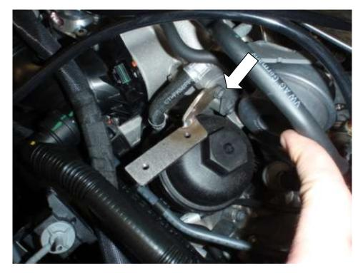
8. Place the solenoid in position and secure to the bracket with the fixings provided.
