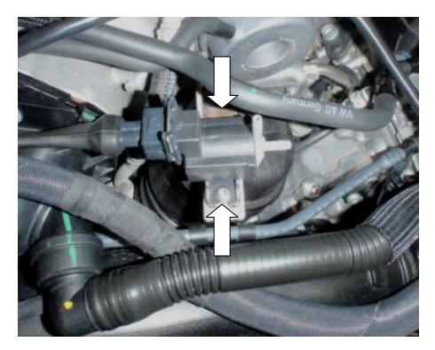
9. Using the silicone vacuum hose supplied connect the boost take-off to the solenoid and the solenoid to the valve. Generic connection diagram shown below:
