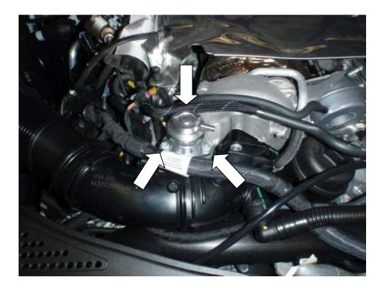
5. Disconnect wiring to the MAP sensor. Using a T30 Torx driver undo 1x screw and remove the sensor from the plastic hardpipe.
