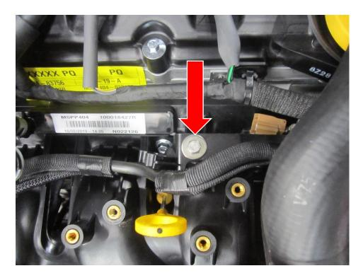
7. Mount the solenoid from the kit as shown in the picture, replace the 10mm fastener you have removed with the M6x20 fastener and M6 washer provided with the kit.
