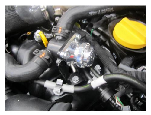
9. The boost pipe on top of the engine needs to be moved over to allow you to run the new silicone vacuum hose for the Forge valve. Undo the 10mm fastener that holds the boost pipe to the engine, then unclip the hose clamp with the use of a flat blade screw driver. You will then be able to pull the boost pipe off the turbo and move it over to the left side of the engine bay.
