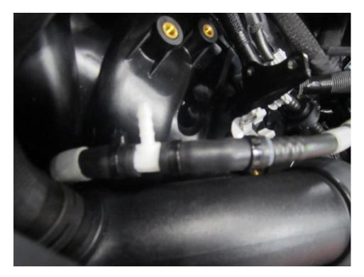
6. There is a 10mm fastener located above the dip stick, move the plastic hose above it to gain access to the fastener. Use a 10mm socket and rachet with an extension and remove the fastener.
