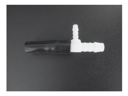
5. Push the one end of the T piece joiner into the rubber side of the brake servo hose, then fit the silicone extension on the remaining brake servo. With that all in place secure with the three larger cable ties provided.
