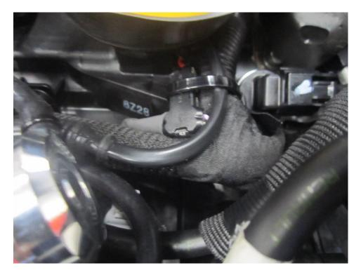
**15**. Refit the boost pipe, push the end of the hose back into the turbo, make sure you hear a positive click when pushing it in, then replace and tighten the 10mm fastener that holds the boost pipe to the engine.
