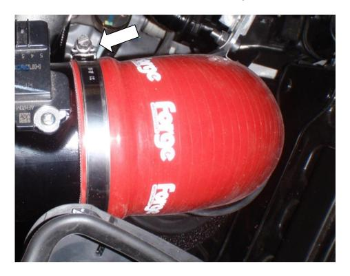
13. Place the P-clip provided around the silicone elbow and using the sheetmetal bracket, 1x M6x16mm Allen cap bolt, 2x 6mm washer, 1x M6 Nyloc, 1x M6x20mm Allen cap bolt, 1x 6mm Penny washer provided secure the hose in position on the bracket shown below.
