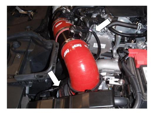
15. Refit the OEM intake scoop and secure in position with 2x OEM bolts. Refit the rubber weather strip clips.
