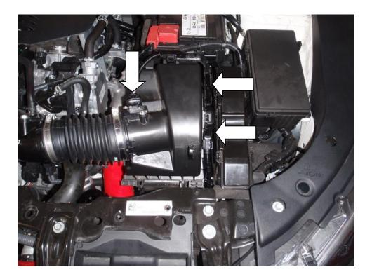
4. Using a Flat-blade screwdriver or 5.5mm socket undo the 2x hose clamps and remove the OEM airbox hose.
