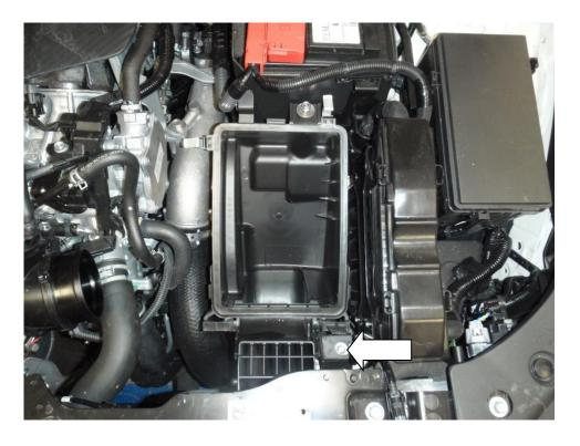
6. Using a Posi-drive screwdriver undo the 2x screw and carefully remove the MAF sensor from the airbox lid.
