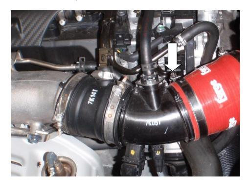
**11.** Insert the Aluminium MAF housing tube into to the open end of the reducing hose and secure with 1x 70-90mm hose clamp. The MAF sensor <u>Must</u> be installed in the orientation shown in the photo below. <u>Failure to do so will cause poor running and EM issues.</u>
