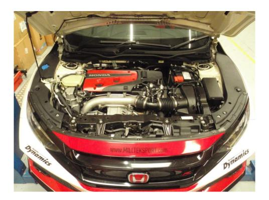
2. Using a 10mm socket and suitable ratchet undo the 2x bolts. Carefully using a trimclip tool or similar unclip the rubber weather strip from the slam panel cover. Unclip the intake scoop from the 2x mounts on the top of the air box and at the neck of the scoop.
