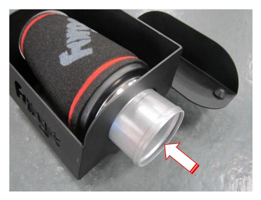
12. At this point, you will be able to install the Forge heat shield. Loosely place one of the larger hose clamps on to the end of the intake hose. Now angle the shield and filter to allow the intake hose to fit to the coupler. Line up the three rubber mounting grommets with the three mounting pegs. When lined up, press the shield down firmly into place. Twist the filter into the desired orientation and secure the alloy coupler with the hose clamp.
