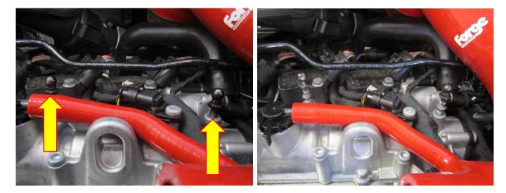
9. Remove the two rubber mounting grommets from the air box, use a flat blade screw driver or trim tool to remove them from the air box. Take your time as they are tightly fitted.
