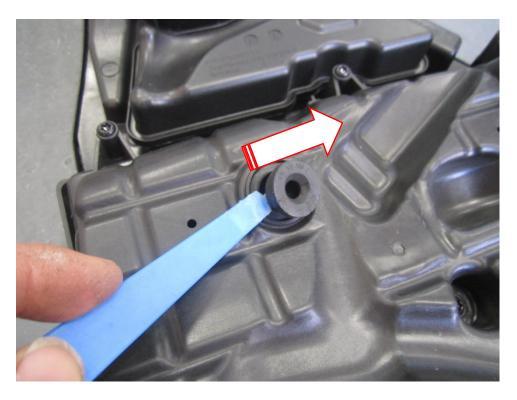
10. Insert the two rubber mounting grommets from the air box and the one supplied with the kit into the Forge heat shield as shown in the picture. You will need to lubricate them to help with fitting.
