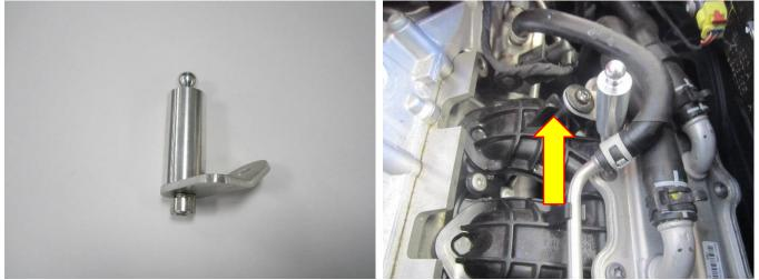
8. Remove the original air box mounting pegs and attach the two steel mounting pegs from the kit on top of the rocker cover
