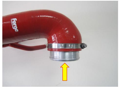
6. Fit the silicone hose at the joiner end to the OE rubber inlet hose and push it in so it's seated snugly. Again, you will need to use a spring clamp removal tool or pliers to secure the joiner to the OE rubber inlet hose. Attach the extended silicone hose to the oil breather as shown in the picture.
