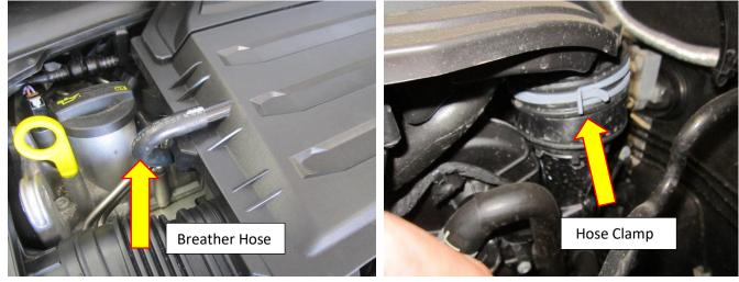
3. Now you will be able to remove the air box from the engine bay, this should just pull out.
