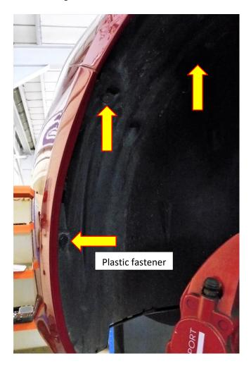
4. Looking from underneath the vehicle, use a T20 Torx drive remove X6 M5 fastener which run along the front of the bumper.
