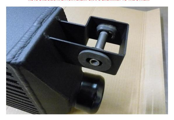
11. Angle the intercooler into position and secure it into position using the original M8 fasteners.
