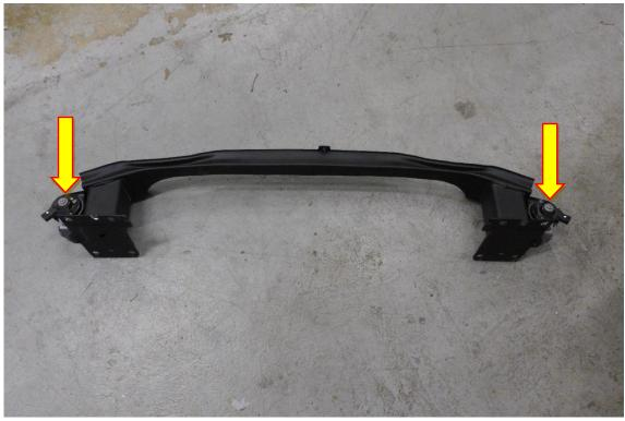
21. Install the Forge crash bar to the vehicle but do not secure into position at this stage.
