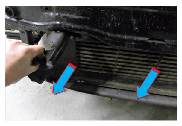
**16**. Using a 16mm socket and rachet with a suitable extension remove 4 x M10 fasteners and using a T27 Torx drive remove 1 x M6 fastener on both sides of the crash bar.
