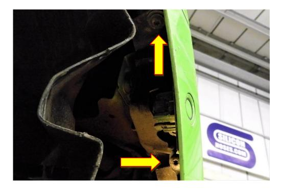
7. Using a T40 Torx driver remove the 3 x fasteners running on the underside of the vehicle.
