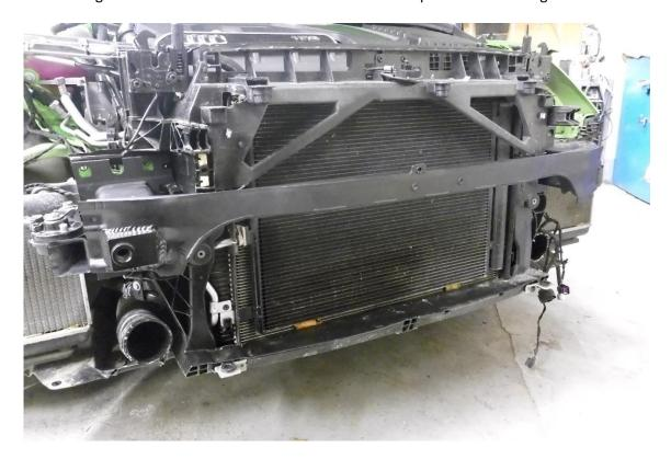
**22.** Take the supplied rubber grommets and machined inserts and fit them to the intercooler as shown in the picture below.
