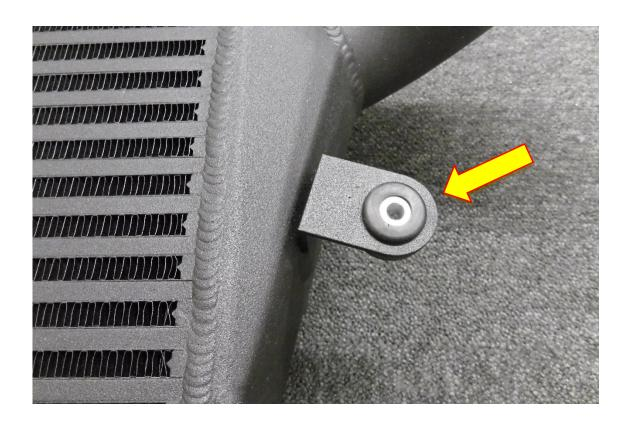
23. Fit the Forge intercooler into place by angling it into position with the lower mounting pegs first then securing the upper brackets using the original fasteners and the supplied penny washers. Attach both boost hoses and tighten both hoses clamps.
