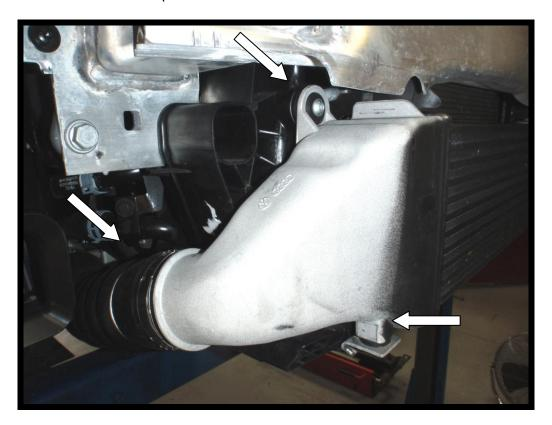
10. Unclip the the air temprature sensor by pushing the small pin out. Be careful not to lose it as it will be reused later, then unclip the wiring from the crash bar.
