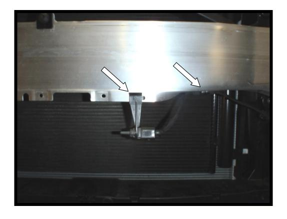
11. Remove the T30 torx and unclip the wiring to the front lights.
