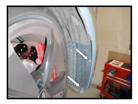
2. Remove the T25 torx screws under the front bumper on each side.
