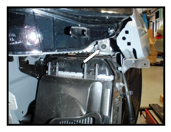
13. Remove the T30 torx and remove the bonnet clip.
