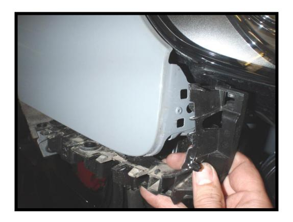
9. Remove the T30 torx from the top and bottom brackets, keeping the bolts and brackets for later use, and undo the hose clamps on both sides.
