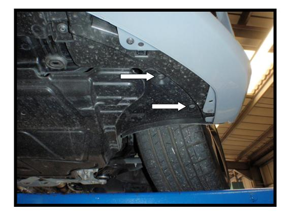
3. Remove the three T30 torx screws at the front of the under tray.
