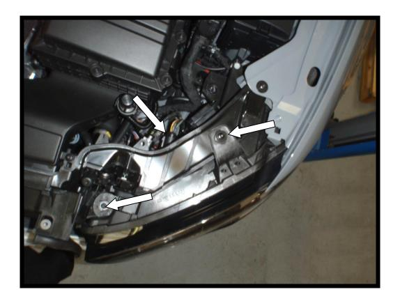
12. There is also a T30 torx at the bottom of the light. Remove this and then the lights are free to remove.
