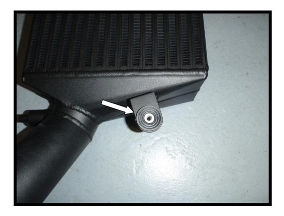
17. Attach the air temperature sensor to the bracket supplied in the kit.
