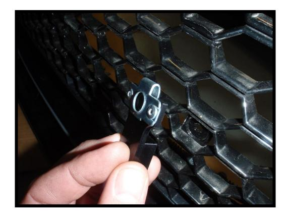
23. The number plate can now be fitted with the quick release bolts.
