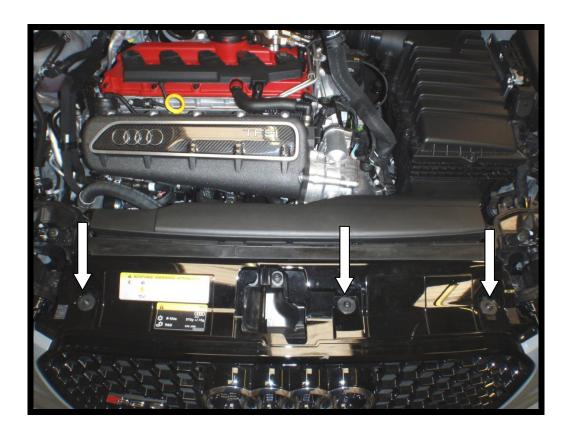
8. Remove the plastic wing clips to enable removal of the lights.
