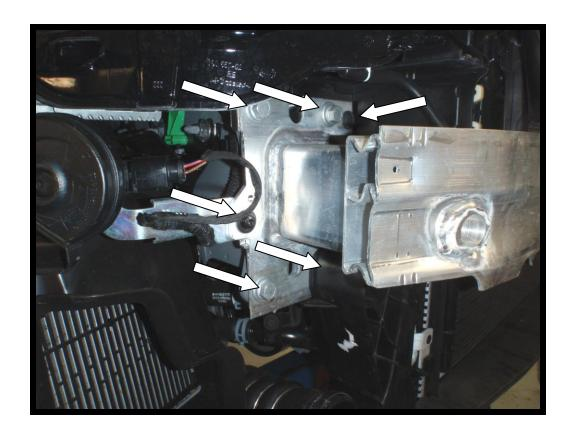
15. Rotate the crash bar and lift upwards and out to remove.
