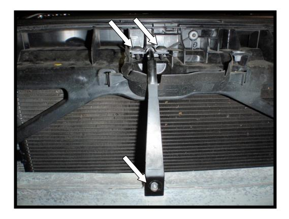
14. Remove the 14mm bolts and T30 torx from the crash bar.
