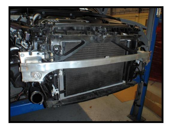
19. Install the new intercooler in reverse order of removal, reuse the brackets and bolts from the OEM intercooler and the large washers and air temperature sensor bracket from the kit.
