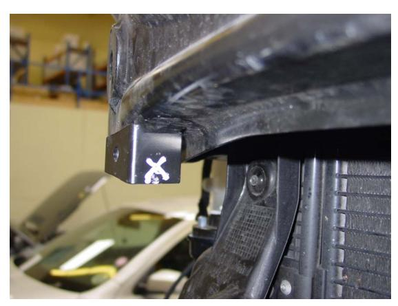
5/ Attach the brackets to the crash bar brackets as pictured below using the nuts and bolts supplied. Then mount the intercooler in to place also but only assemble the fixing nuts and bolts loosely at this stage.
