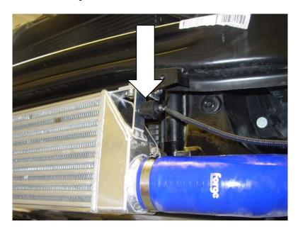
9/ Before the bumper can be refitted you have to remove the lower plastic brace panel as shown below. This can be simply removed from its plastic fixings with a sharp knife and a drill. You may also need to remove the two plastic prongs on the edge of the foglight covers nearest the intercooler as they can foul the intercooler hoses on certain models.
