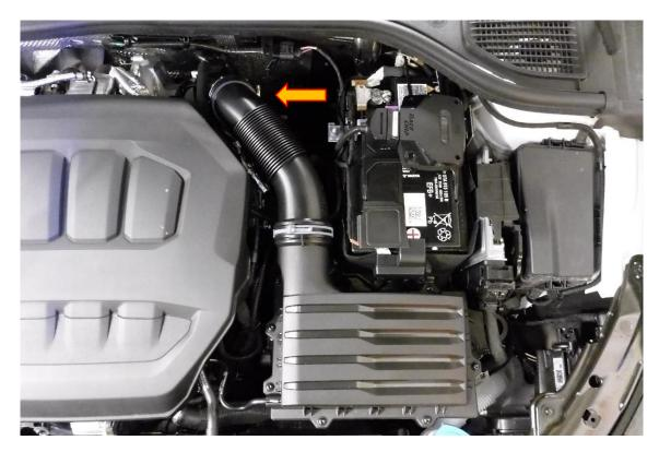
2. Disconnect the vacuum hose attached to the air box, this simply pulls off. The air box and intake pipe will all lift out as one, to do this pull sharply in an upwards motion to release the air box from its rubber mounting points.
