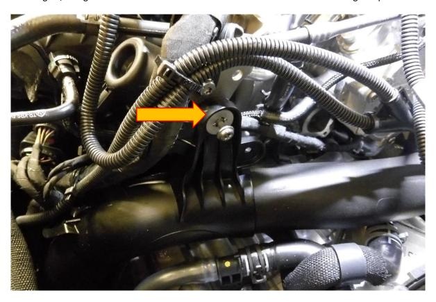
4. Using a 7mm socket or suitable hose clamp drive loosen the two hose clamps attaching the rubber boost hose to the turbo muffler, you can now remove the hose from situ.
