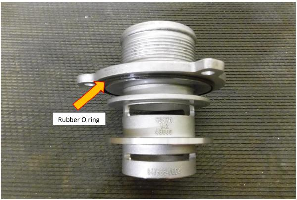
6. Fit the O-ring removed from step 5 to the Forge Motorsport Muffler delete, Now using the fasteners removed in step 5 fit the FMMD6 in the same orientation as the original turbo muffler. Tighten with a T30 torx drive and secure in position.
