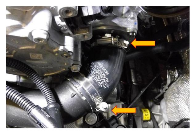
5. Using a T30 torx drive remove the 3 fasteners attaching the muffler to the turbo, the muffler can now be removed from situ. When removing be cautious not to lose the rubber O-ring that is housed on the mating face.
