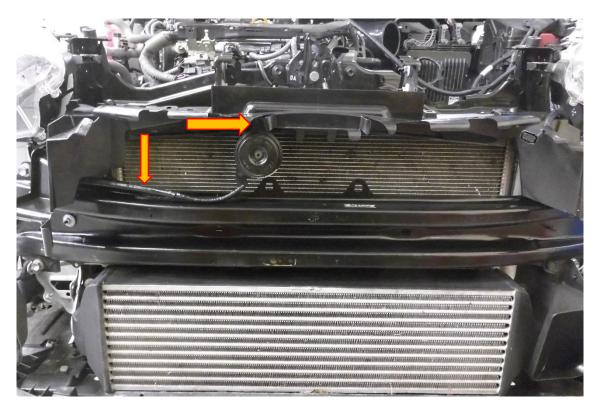
12. Using a trim tool remover or flat bladed screwdriver remove the 2 X plastic retaining fasteners attaching the plastic slam panel trim using a trim tool or flat blade screwdriver.. With both fasteners removed the trim can be removed from situ.
