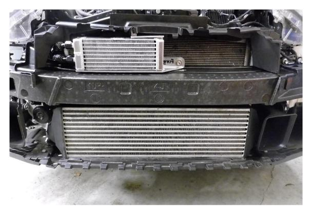
22. Add half a litre of the appropriate grade engine oil to your vehicle to compensate for your new Forge oil cooler. Now start the engine, get it to full running temperature and check for oil leaks, if you do find any leaks; wait for it to cool down and tighten fittings accordingly.
