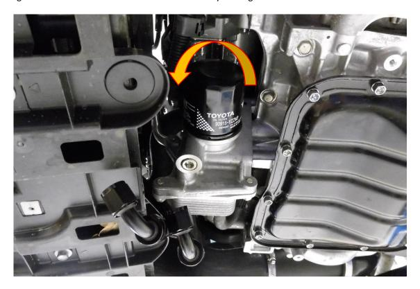
19. Offer up the oil take off plate where the oil filter used to be in the orientation illustrated below, make sure the rubber O ring side is facing towards the engine and secure it in place with the threaded extension supplied. Clean the sealing face for the oil filter, smear a small amount of clean oil on to the sandwich plate O -ring. Use a 26mm extended socket or 26mm spanner to tighten the threaded extension fully, now fit the oil filter onto the threaded extension.
