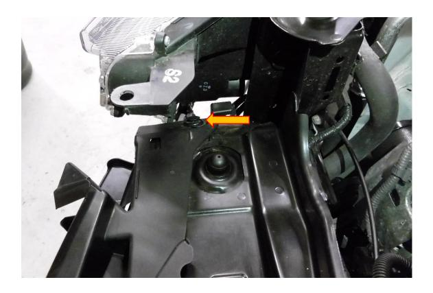
**13**. Unplug the wiring loom connected to the horn. Using a 12mm socket and suitable ratchet remove the m8 fastener attaching the horn to the slam panel to allow you to remove the horn.
