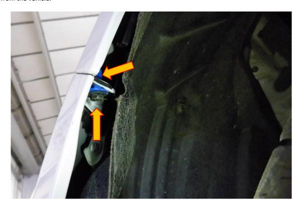
8. Using a plastic trim tool open up the black retaining clips to allow the edge of the bumper to come away from the wing. Use masking tape to avoid marking the paint work. When both sides are free from the wings carefully rest the bumper and unplug both fog light wiring looms by depressing the tab on the plug.
