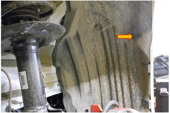
7. Using a 10mm socket and ratchet remove the M6 fastener on both sides of the bumper, the plastic retaining clip also needs to be removed. This simply pushes out of its housing. The bumper can now be pulled away from the vehicle.
