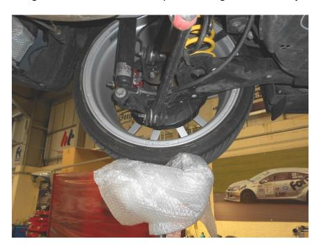
3. Using an 8mm socket, short extension bar and suitable ratchet undo 3x bolts and remove the plastic guards on both sides.
