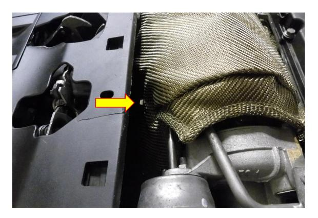
8. Using a 10mm socket and ratchet with extension remove the lower M6 fastener attaching the bonnet catch.
