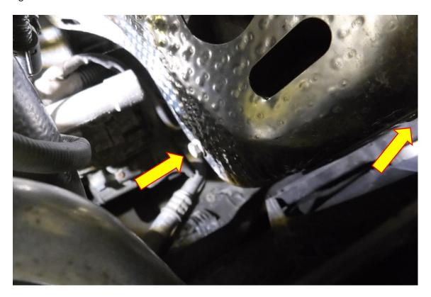
4. Un-plug the lambda probe loom.
