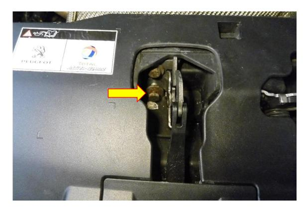
9. Take one of the original 3X M6 fasteners which was removed in Step 2 and the M6 20mm washer from the FMTUBL14 kit and replace the M6 fastener removed from the bonnet catch.
