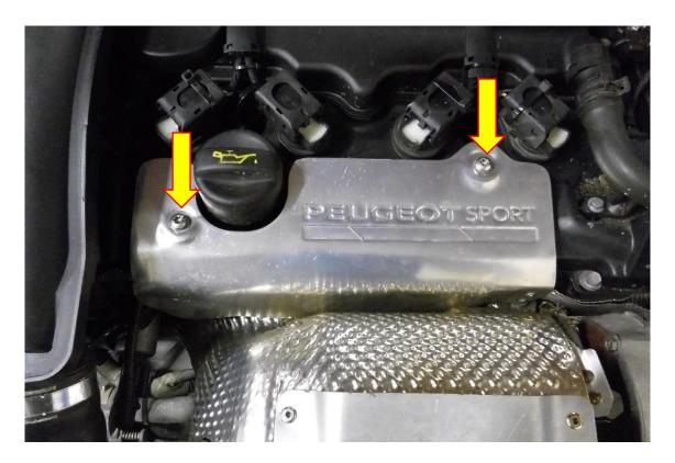
2. Using a 10mm socket and ratchet remove the 3X M6 fasteners attaching the top half of the turbo heat shield to the engine.
