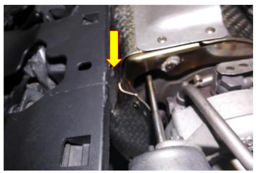
6. Place the Forge turbo blanket over the turbo, pass the lambda probe loom through the large hole. Using a 5mm Allen key attach 3X M6 fasteners and M6 penny washers to top of the turbo blanket securing it to the engine and 2X M6 fasteners and M6 penny washers securing the bottom front of the turbo blanket to the down pipe.
