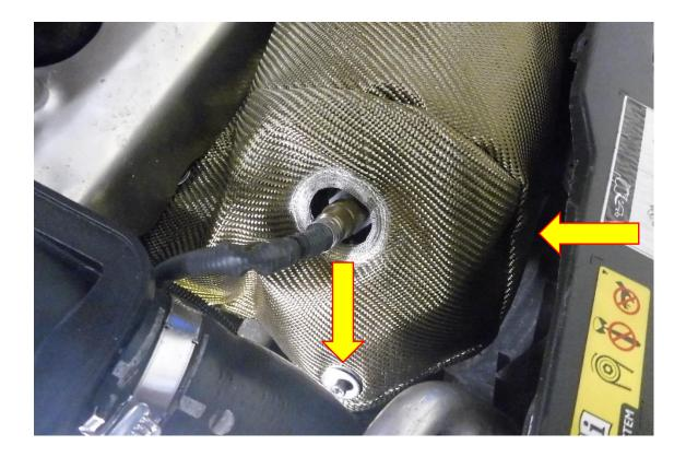
7. Using a 10mm spanner attach the M6 flange nut from the FMTUBL14 kit.
