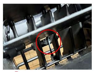
Be sure middle slat aligns with fork to retain horizontal control
