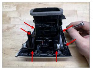
Release 6 clips on sides and bottom of vent
