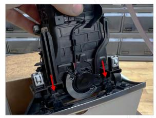
Slide vent housing down onto trim assembly, partially inserting bottom 2 clips (But do not fully seat yet)
