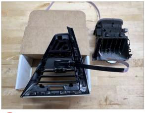
While keeping display cable in vent housing as shown, lay slat assembly and display into trim (Be sure all pegs are aligned correctly)
