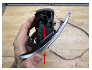
Finish snapping trim and housing together, fully seating all 8 clips
