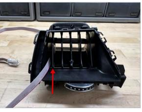
Feed cable through vent against left side of housing. \*OPTIONAL - Left vertical slat can be removed for extra cable clearance
