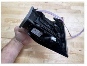
Tightly fold display cable around back of housing and pinch foam back into place
