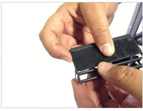
In the side vent slat retainer bars install the P3Cars gauge into the existing vent slat holes.
