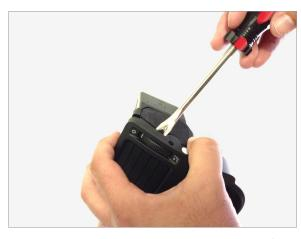
With a smooth thin trim tool or thin flat head screw driver release the round recessed clip on the right.
