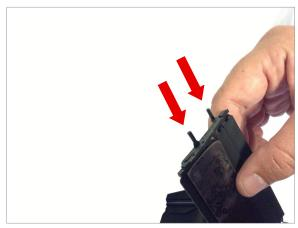
Insert these into the key way inside the roller from frame 10. BE sure that the rear flap is in the closed position as the vent slats and rear flap need to move in synchronicity.
