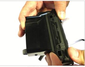
Clip top clips insuring that the P3Cars display protective covering is NOT stuffed behind facia.
