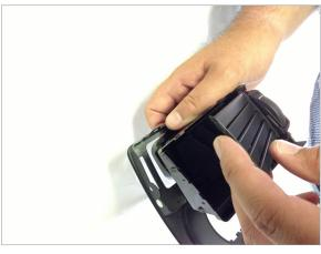
Starting from the LEFT side of the vent remove the vent slats
