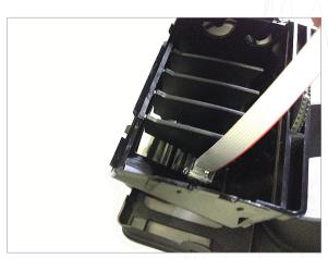
Feed cable in left side of vent housing against bottom left side of vent interior.
