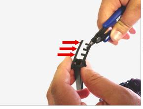
With a sharp pare of snips clip the three protruding keepers on the keeper rail.
