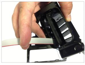
Manually open rear flap and slide cable out bottom left then manually close flap against it.
