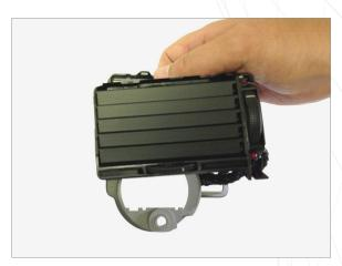
Rotate facia trim to the rear underside of vent housing leaving vent slats exposed. PLEASE NOTE you will need to leave the RIGHT side roller, front slats and rear flap in this position for ease of reassembly
