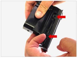
On the left of the vent housing pull facia away from clips and release top left clip.
