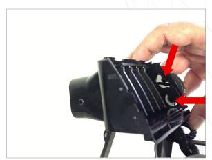
Re-attach the vent face, starting at the bottom with the 2 circular clips.
