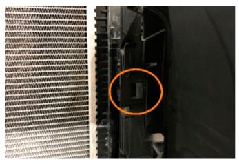
**11.** Remove the upper passenger side (LHD) rock guard tab with a cutoff tool.
