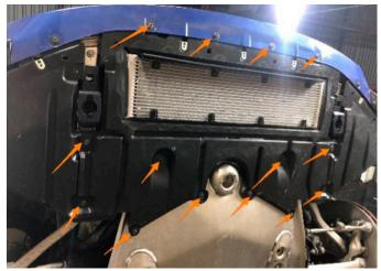
2. Remove the front bumper cover. Refer to the factory workshop manual for specific details.
