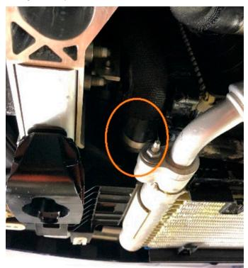
**5.** Remove the upper radiator cover bracket. Remove the 6x 13mm bolt, 5x black T30 bolts, and 4x silver T40 bolts. Next, remove the push pins from the front of the bracket. Once complete, remove the hood latch cable from the tabs and remove the upper radiator bracket from the vehicle.
