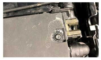
**18.** Reinstall the upper radiator bracket. Remember to reinstall the hood latch cable in its proper location to ensure that the hood will open properly.
