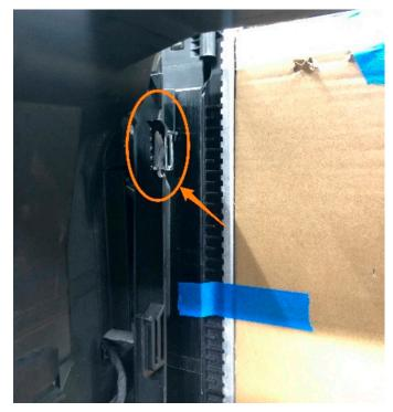
**12.** Install the Mishimoto heat exchanger into the vehicle. It may be helpful to rotate the heat exchanger clockwise (facing the front of the vehicle) in order to get the lower outlet into its spot in the radiator support plastic.
