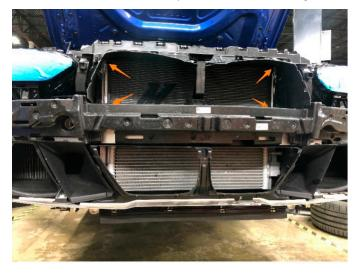
**16.** (Manual vehicles only) Remove the T30 screw securing the factory lower rock guard to the vehicle and remove from the vehicle. Install the included lower rock guard with the factory screw.
