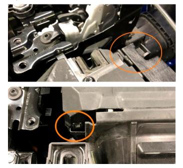
8. Remove the upper heat exchanger hose by removing the clip and pulling the hose away from the heat exchanger.
