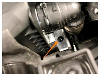
**14.** Install both the inlet and outlet hoses on the Mishimoto heat exchanger. You should hear an audible click when they are fully seated.
