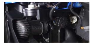
13. Loosen the clamp securing the cold-side hose to the intercooler end tank. Then, separate
