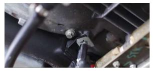
17. Loosen the clamp holding the hot-side pipe to the turbo, but leave the pipe there for now.(1x worm gear clamp)
