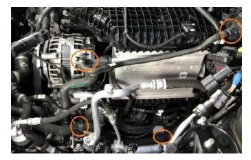
**15.** Remove the intercooler coolant line as well as the auxiliary water pump inlet hose from both the intercooler as well as the auxiliary water pump. Remove the 1x 10mm nut from the auxiliary water pump. Remove the electrical connector from the back of the auxiliary water pump and remove the pump from the vehicle.
