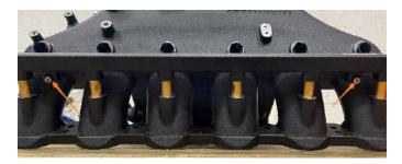
**47.** If you are using port injection, install the remaining fuel line into the fitting at the end of the fuel rail and tighten with a -6AN wrench.
