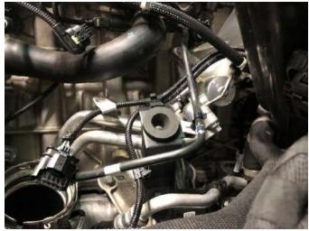
**39.** Remove the EVAP hose connected to the EVAP solenoid that sits under the intake manifold. Using a heat gun, heat up the ends of the hose and remove both fittings. This can also be accomplished by cutting the end of the hose with a razor blade, however, it may risk damaging the o-ring on the end of the fitting and the line will not be reusable. [Image on top right]
