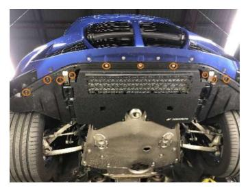
**04.** Remove the 14x 10mm screws securing the undertray to the vehicle and remove the undertray (Mishimoto Skid plate shown).
