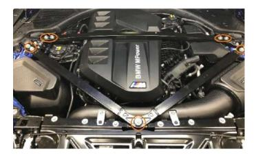
**10.** Remove the front turbo intake. Remove the 2x push clips on the radiator support. Remove the quick disconnect at the turbocharger inlet and remove the intake box and intake pipe from the vehicle.
