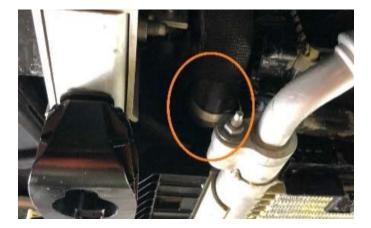
**09.** Remove 4x 15mm nuts securing the cross brace to the vehicle and remove. Remove the 4x 15mm nuts and 1x 13mm bolt securing the V-brace to the vehicle and remove. Remove the plastic engine cover by pulling up.
