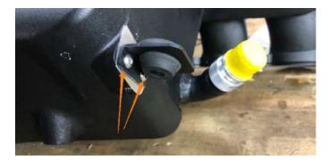
**30.** Install the EVAP fitting into the port near the throttle body with 1" or 25mm socket. Install the included -10AN plug on the front of the intake manifold plenum. These are o-ringed connections, so they do not need to be very tight. We recommend 20ft-lbs or less. If you are installing on an X3/X4, these two fittings will likely be switched. (Images on top right)
