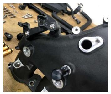
**33.** Install the included engine cover mount into the hole shown with a 13mm wrench. This step may be skipped if not planning to run an engine cover.
