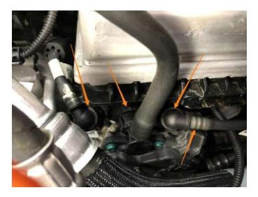
17. Remove the 10mm nut holding the EVAP line into the top of the manifold. Disconnect the EVAP sensor electrical connector and unclip the pinch clip holding the EVAP sensor into the EVAP T fitting. Then, remove the EVAP line from the metal bracket on the intake manifold. Disconnect the MAP sensor electrical connector and remove the clips holding the MAP sensor wiring harness in place.
