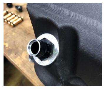
**31.** Install the lower manifold support fitting in the bottom plenum of the manifold. It can be tightened using a 13mm wrench as shown in the picture below.
