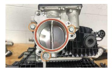
27. Install the throttle body onto the Mishimoto manifold using the included 45mm long M6 bolts. We suggest putting a dab of blue Loctite onto the bolts onto the threads of the bolts. Tighten each of the 3 bolts to about 4-5 Nm and then go back and tighten the bolts to 12-14 Nm in a circular pattern. Then, install the throttle body adapter to the throttle body with the 3x factory bolts. Torque to 8-10 Nm.
