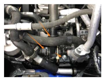
16. Remove the lower EVAP connector and the two throttle body coolant lines to gain access to the throttle body electrical connector.Disconnect the throttle body electrical connector. (Image on top right)
