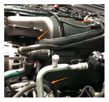
**43.** This manifold is capable of using both the factory rubber green O-rings or the included fiber gasket. We have provided the fiber gasket as it has thermal insulating properties to prevent heat transfer from the cylinder head to the intake manifold. At this time, remove the factory green o-rings from the factory manifold and install them onto the Mishimoto Manifold OR install the included gasket onto the pins on the Mishimoto manifold. **USE THE O-RINGS OR THE GASKET BUT NOT BOTH!**
