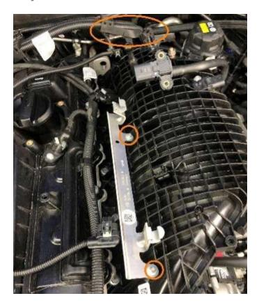
**19.** Lift up on the auxiliary coolant reservoir to remove it from its lower bracket in order to make room to reach the rear coolant hose for the intercooler. Remove the spring clip and pull the hose away from the intercooler to remove.
