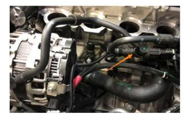
**40.** Install the fittings from step 37 into the included hose (MM4624-02, the shorter or the two included hoses) and secure with 2x of the included worm gear clamps. Try to clock the fittings similar to how they are positioned in the vehicle. Reinstall the hose on the EVAP solenoid that sits under the intake manifold.
