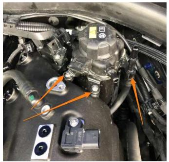
**50.** Connect the EVAP hose with the EVAP sensor to the EVAP hose Tee fitting. Install the EVAP hose into the manifold and secure with provided 12mm long M6 button head flanged bolt. Make sure that the EVAP hose is clipped into the metal clip attached to the bracket. Connect the MAP sensor electrical connector and secure into the wire loom clips on the supplied brackets. (Image on next page)
