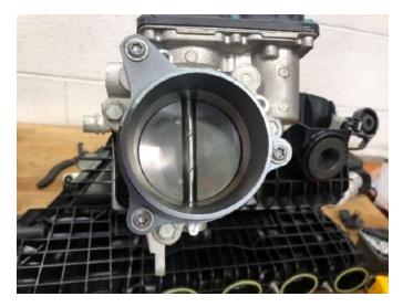
**26.** Remove the 3x 10mm bolts that hold the throttle body to the stock manifold. Make sure that both orange O-Rings stay with the throttle body. (Image on top right)
