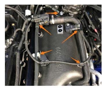
**51.** Reach under the manifold and connect the charge pipe to the throttle body adapter. This may be easier from underneath the vehicle with the undertray removed.
