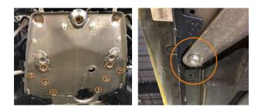
**07.** Remove the main cooling system reservoir cap. Then, disconnect the coolant lines at the auxiliary radiators in front of each wheel well. Remove the spring clip from the fitting and pull away from the radiator. Drain one at a time to avoid making a mess. (Note: If attempting installation on an X3/X4, one of the auxiliary radiators is used for the secondary (intercooler) cooling system).
