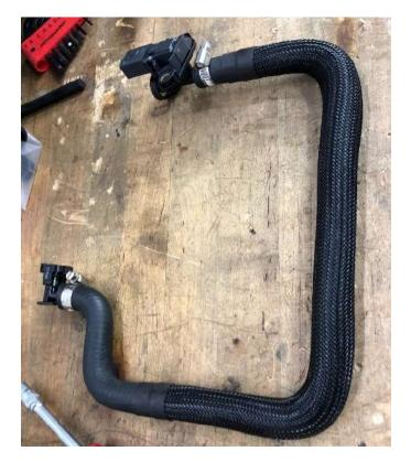
**42.** Install the fitting side of the hose on the EVAP solenoid that sits under the intake manifold. This hose will now route towards the front of the car and around the intake manifold, instead of under the manifold. This hose will be routed on top of the hose that was assembled in steps 37 and 38. We have included a picture of the installed manifold for reference.[Image on top right]
