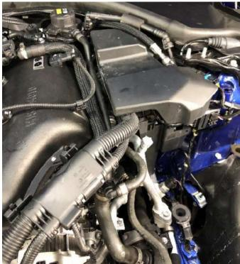
**55.** Fill the auxiliary and main coolant reservoirs with coolant. We suggest using a vacuum filling system for the best results. Once full, make sure to check for leaks at all the coolant connections that were removed during the installation process.
