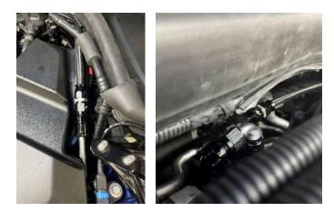
**24.** Install the last line with the two 90° hose ends on the remaining end of the T-fitting. Leave the other side loose as this will go into the fuel rail.
