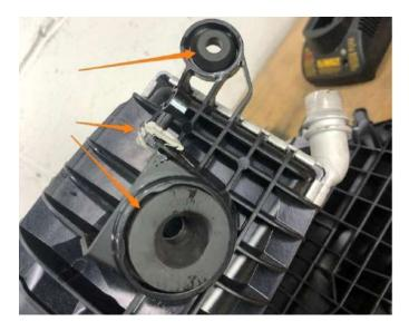
**29.** Install the 90° bracket with the smaller grommet (MM2428-04) on the manifold with the included 6mm long M4 button head screws.
