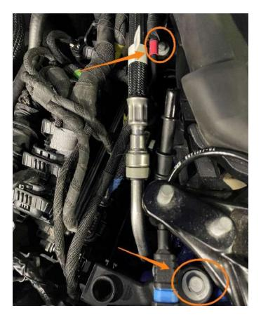
**13.** Remove the engine electrical harness off of the manifold and push the harness to the side.
