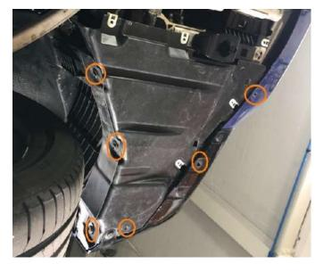
**06. (Optional)** Remove main aluminum skid plate from the vehicle. This is not 100% necessary for the removal and installation of the intake manifold/intercooler, however, it will provide additional access to the underside of the engine and will make it significantly easier to retrieve any dropped bolts or sockets during the installation process.
