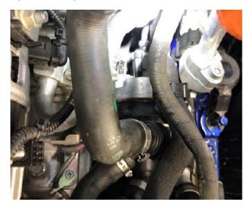
**53.** Reinstall the coolant line that runs from the outlet of the water pump to the intercooler/intake manifold. Reinstall the smaller line that connects from the fitting of the intercooler coolant line to the auxiliary coolant reservoir.
