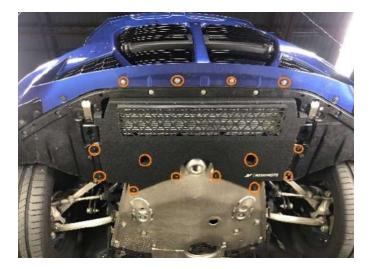
**05.** Remove 6x 10mm screws (per side) holding the side undertrays to the vehicle and remove from the vehicle to gain access to the auxiliary radiators. If you do not plan on draining the main cooling system, this is not necessary. We suggest draining the main cooling system as the throttle body coolant lines must be disconnected to remove the intake manifold/intercooler from the vehicle. (Image on next page)
