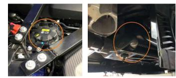
**08.** Remove the cap for the auxiliary cooling system reservoir at the rear of the intake manifold/intercooler. Remove the spring clip from the quick connect fitting at the bottom of the heat exchanger and drain the auxiliary cooling system.
