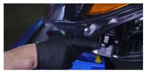
3. Remove the pop-clips that secure the undertray to the stabilizer bar. (2x pop-clips)
