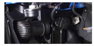
13. Loosen the clamp securing the cold-side hose to the intercooler end tank. Then, separate the connection. (1x worm gear clamp)
