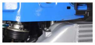
25. Secure the bottom of the intercooler with the original hardware.
