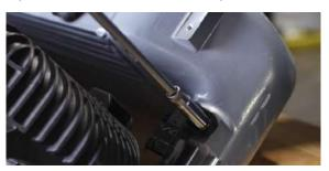
22. Slide the provided clip nuts onto the intercooler's lower brackets.
