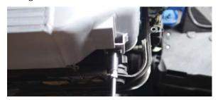
26. Install both diversion plates included in your kit to the bottom edges of the intercooler. Be careful not to overtighten these bolts during installation.
