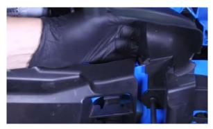
18. Pull the rest of the ducting at the sides of the intercooler from behind the bumper bar.
