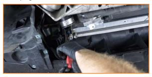
15. Separate the transmission cooler lines. (2x T25 torx bolts)
