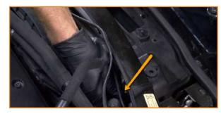
6. Disconnect the electrical fan connector. Depress the tabs at the sides to free the connector.
