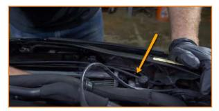
Separate the upper radiator hose from the radiator by releasing the clip on the hose connection. (2x spring clips)
