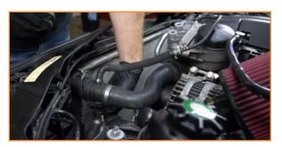
10. Separate the lower radiator hose from the radiator by releasing the clip on the hose conneciton. (1x spring clip)
