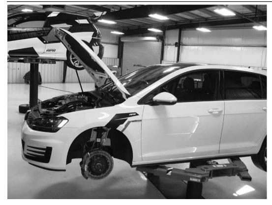
52) Support the car on a lift or jackstands. Raise the hood and remove the engine cover.
