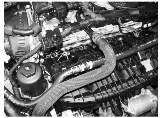
88) Remove the covering you had protecting the intake ports on the cylinder head. Carefully place the intake manifold back towards its mounting location on the cylinder head. It may be necessary to remove the oil filter housing to get the manifold fully in place.
