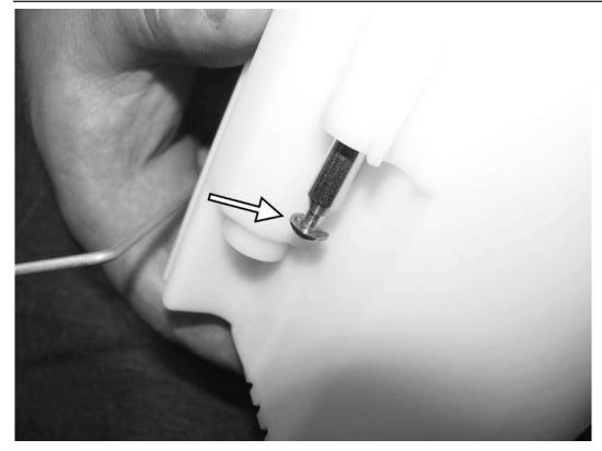
12) On a clean work area, remove the circlip from the bottom of the spring loaded rod on the bottom of the fuel pump. Do not lose this circlip, as it will be reused. Lift the spring loaded top of the fuel pump off the fuel pump basket and set aside.
