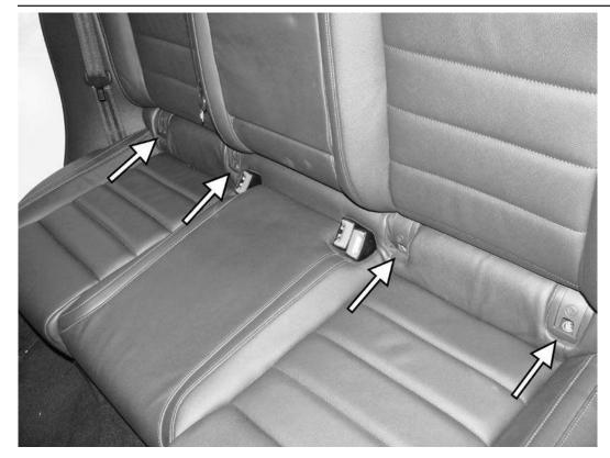
2) Remove the four covers over the child seat locking points by pulling the plastic covers away from the seat bottom.
