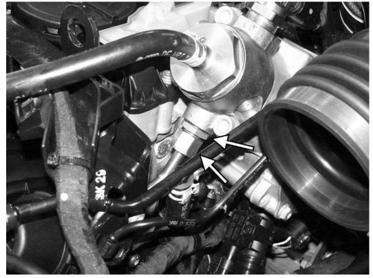
70) Holding the brass fitting in the bottom of the HPFP with a 21mm wrench, use a 17mm wrench to loosen the fuel line from the brass fitting. Use a rag around the connection while breaking the connectin loose to prevent gas from spraying or dripping.
