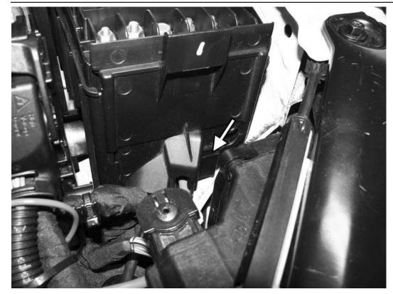
130) Remove the top cover to the underhood fuse box. Pull the holding tab out towards the front of the car, and lift up to remove the front panel of the fuse box.
