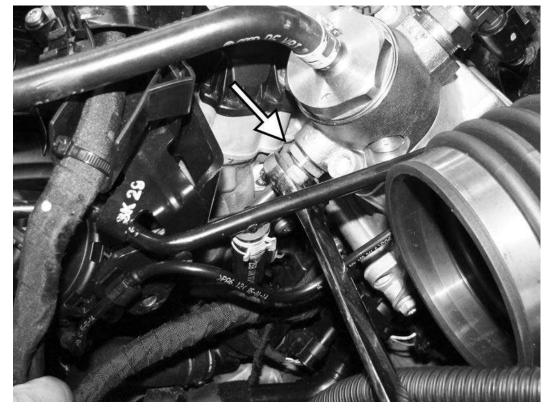
96) Holding the brass fitting in the bottom of the HPFP with a 21mm wrench, use a 17mm wrench to tighten the fuel line to the brass fitting. Also reinstall the one T30 screw that holds the fuel line in place.
