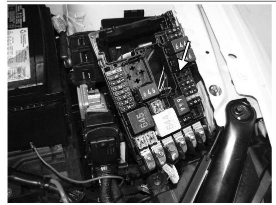
132) Fully lift the fuse plate in order to access the back side of it. Route the red power wire from the APR harness along with the other factory power wires underneath the front of the fuse box. Finally, locate the empty fuse opening, on the left side of the fuse box, at the back of the row of fuses.
