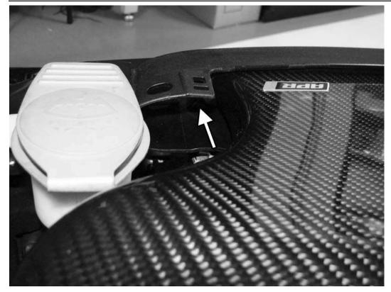
136) Install the APR intake back to the front of the core support by sliding the left side of the intake into the slot on the core support. Then install the original screw into the right tab on the intake to support it.
