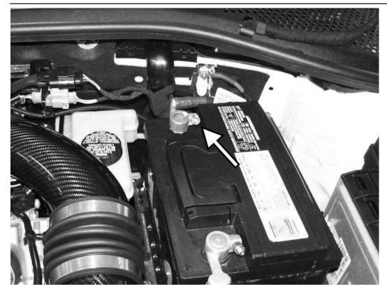
138) Reconnect the negative battery terminal and secure the 10mm nut holding it in place.
