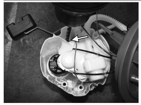
16) Locate the last mounting hole on the opposite side of the two holes just drilled. Drill this hole all the way through carefully with the 6.5mm drill bit.
