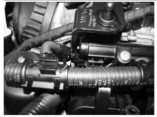
102) Install the electrical connector from the APR harness to the #1 fuel injector. Tuck the wiring for the connection to the intake manifold runner flap position sensor under the intake manifold. Also connect the electrical connector on the APR harness to the fuel pressure sensor on the fuel rail.
