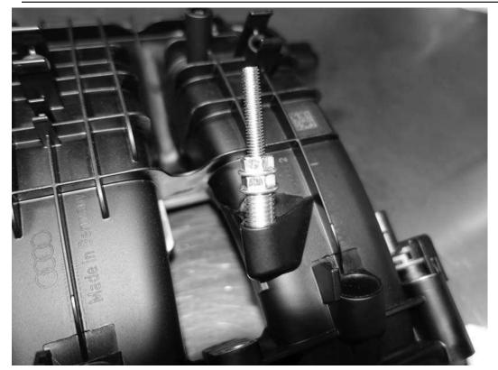
80) Place the supplied threaded inserts onto the previously drilled holes. Loosely thread the supplied stud into the insert at least 10mm. Install the two 10mm nuts all the way down to the top of the insert, and double nut the two nuts together so that you can turn the entire assembly as one.
