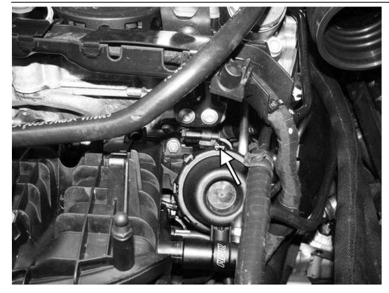
64) Disconnect the electrical connector to the camshaft position sensor located on the left side of the engine, behind the intake manifold runner flap actuator.
