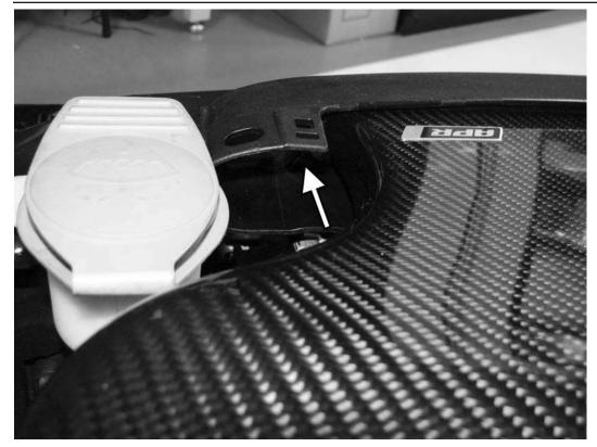
54) Remove the screw holding the APR intake to the back side of the radiator core support. Slide the intake towards the left side of the car to separate it from the core support.
