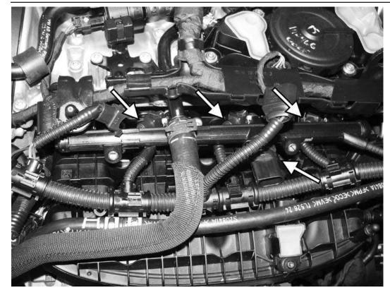
100) Connect the APR harness to port injectors #2, #3, and #4, leaving the #1 (the far right) injector injector unplugged. Install the fuel pressure sensor in the fuel rail with a 27mm wrench or deep well socket and torque to 132 in-lb (15Nm).
