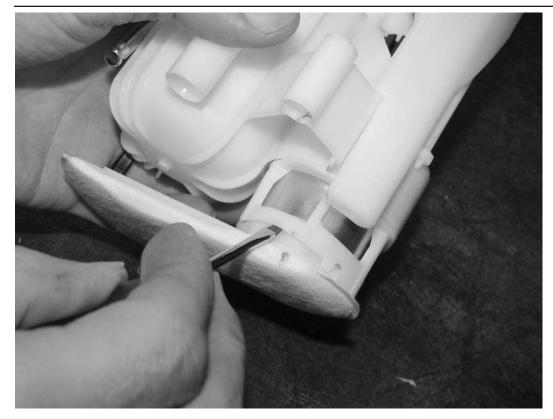
20) Using a small screwdriver, carefully pry both sides of the fuel pump sock awat from the fuel pump assembly.
