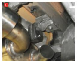
A) After you have removed O.E exhaust you will need to remove the two rear valve motors (Right hand side and left hand side). remove 6 x 8mm nuts from both sides (3 on each valve, keep safe as you will need them to bolt the electronic valve motors to Scorpion Exhaust).
