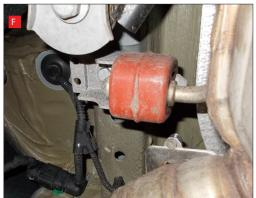
F) When fitting the Scorpion rear silencer (605AU) the rear most mounting bracket's need to be rotated through 180 degrees to allow correct fitment. This needs to be done on both sides of the car.
