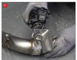
B) Lift up the motor. You will now be able to see the torsion spring (This must stay on the electronic valve motor to work with Scorpion Exhaust DO NOT REMOVE SPRING AND DO NOT TURN MOTOR)
