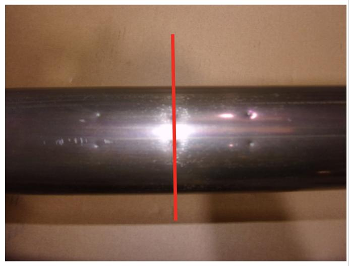
To make it easier to cut the exhaust we reccomend remoiving it from the car. Find the 3 pairs of indents and use the middle pair to mark out the cutting line. Cut along the line and de-bur the edges. Re-fit the original GPF and fit the Scorpion GPF-back following the line diagram above.
