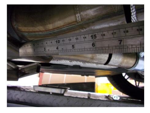
To fit this system the original exhaust requires cutting.
