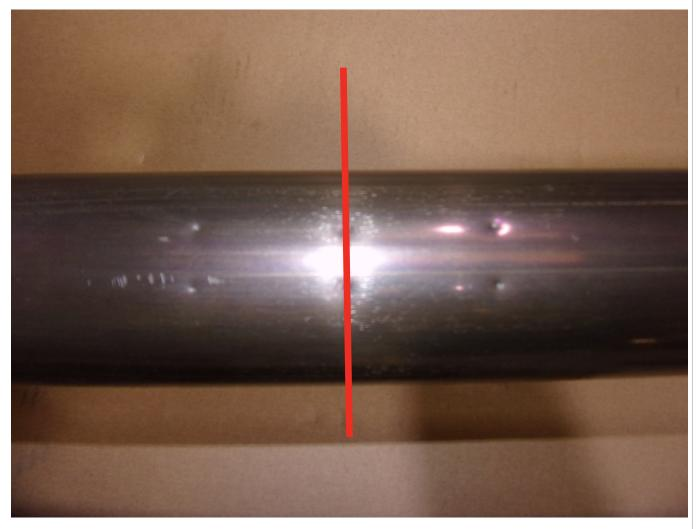
To make it easier to cut the exhaust we reccomend remoiving it from the car. Find the 3 pairs of indents and use the middle pair to mark out the cutting line. Cut along the line and de-bur the edges. Fit the Scorpion GPF delete and fit the original GPF-back or the Scorpion GPF-back system.
