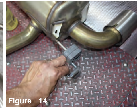
Figure 14 Remove the Rear Factory hangers.
