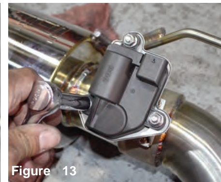
Figure 13 Once the shaft and spring are seated correctly. Tighten all nuts and secure. If the motor shaft is not seated correctly with spring it will not work properly with sport mode function.
