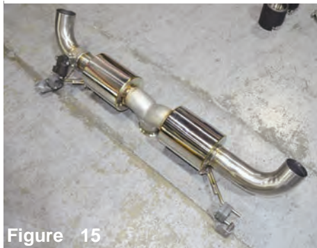
Figure 15 Re-install the hangers to the injen rear muffler assembly.
