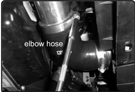
20. Adjust for fitment. Make sure all connections are properly secured. Re-route harness or lines. Re-adjust if necessary. Tighten all clamps using 8mm nut driver or ratchet. Tighten and secure the bracket using 10mm socket or wrench.
