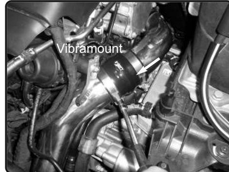
19. Connect the hose and adjust. Make sure the hoses are properly adjusted and clamps are behind the bead. This will prevent hoses popping off the pipe. Secure the bracket using provided washer and nut.
