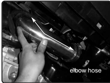
18. Install the lower intercooler pipe into the vehicle. Position to the upper intercooler pipe and bracket to the vibramount.
