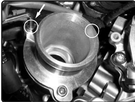
12. Secure the adaptor using original screws from step 9.
