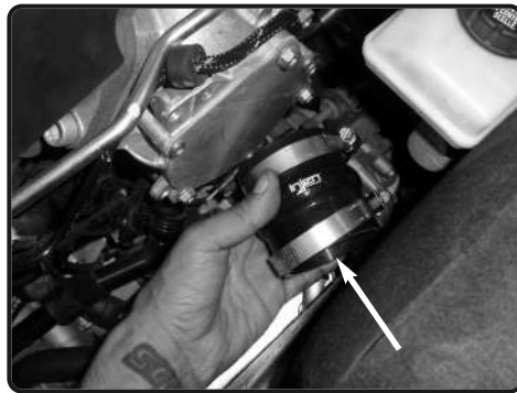
14. Install the provided 2-1/2" hump hose with clamps to the turbo adaptor.
