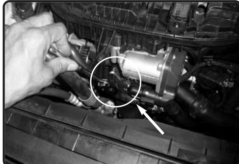
21. Loosen the clamp on throttle body using 7mm nut driver or ratchet.
