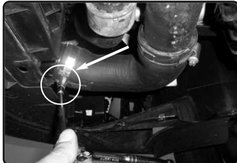
22. Loosen the clamp on intercooler using 7mm nut driver or wrench.
