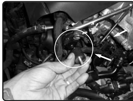
13. Install the M6 vibramount to the original mounting point from step 4.
