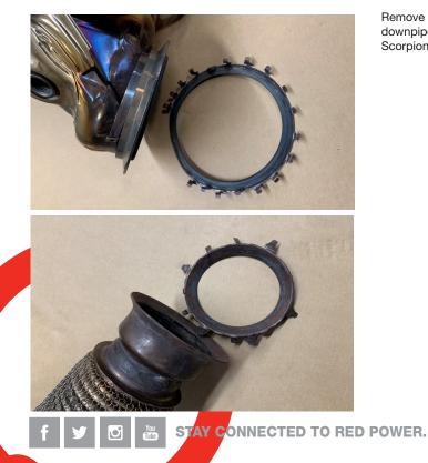
Remove the original gaskets from the original downpipe as they are required when fitting the Scorpion downpipe.
