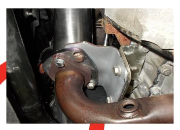
The Mounting bracket replaces the original mounting bracket. Bolt the flange of the downpipe to the mounting bracket. Bolt the flange of the Scorpion or original cat-back system to the flange of the downpipe as shown in the picture.
