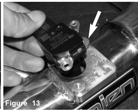
Figure 14 Secure MAF sensor using provided M4 button head screws. Tighten using 2.5mm allen key.
