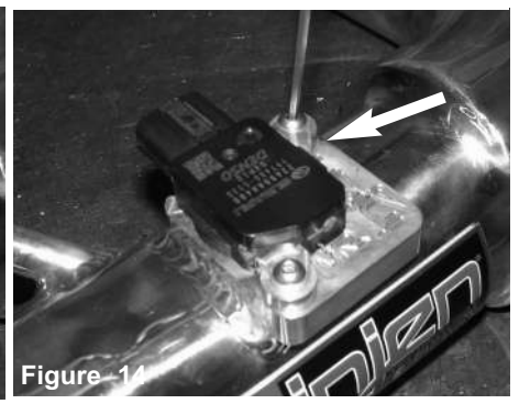
Figure 13 Install the MAF sensor into the intake tube.
