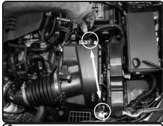
**6.** Loosen the two 10mm bolts holding in the stock air box.
