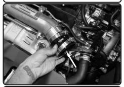
**35.** Install the provided step hose with clamps to the turbo.
