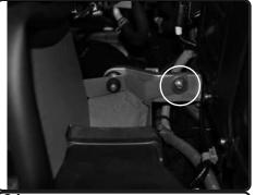
**31.** Secure the bracket using propvided M6 hex screw and fender washer. Secure and tighten using 10mm socket or wrench.
