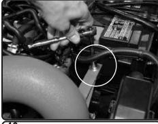
**40.** Secure the bracket using provided M6 nut and fender washer.
