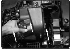
**10.** Lift up and remove the airbox.
