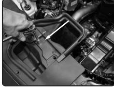
**32.** Secure the scoop and push clips from steps 2-3.
