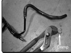
**19.** Remove clamp from the coolant line.
