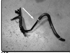
**18.** Remove the complete Crankcase/coolant hardline from fitting out of vehicle
