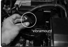
**36.** Install the provided M6 vibramount to the OEM airbox mounting bracket. Secure and tighten.
