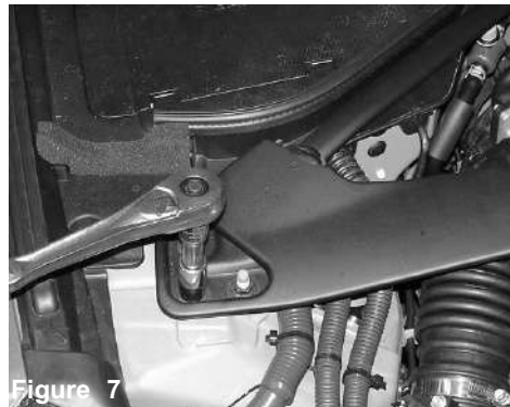
Figure 7 Passenger side strut tower- Loosen and remove two 14mm bolts and one 14mm flange nut from the stabilizer bar.
