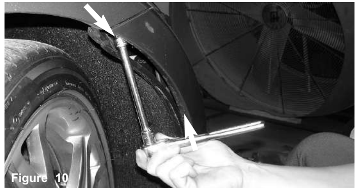
Figure 10 Remove the 10mm bolt located on the passenger and driver side upper wheel well.
