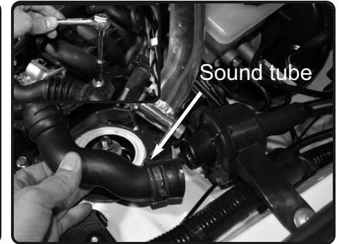
3. With pliers, bull back the line from sound tube. Loosen the 10mm screw holding in the sound tube.
