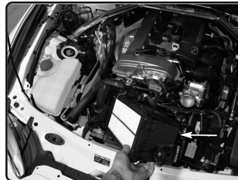
6. Now carefully remove the bottom air box assembly by pulling up from vehicle.
