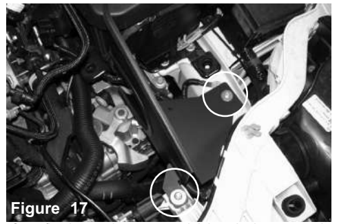
Figure 12 Install the vibramount to the threaded insert from step 5. Secure and tighten.
