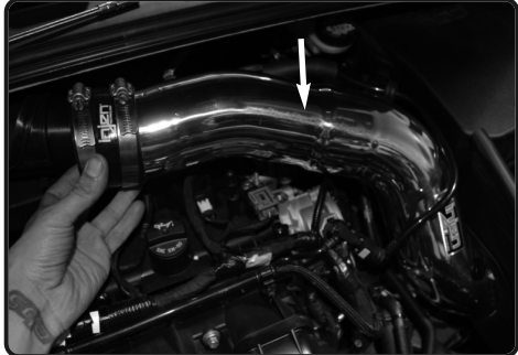
20. Install the intake and position the bracket to the stand off stud.
