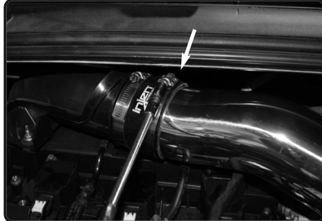
21. Tighten the clamp using 8mm nut driver. Position for best fit and make sure tube is not touching anything.
