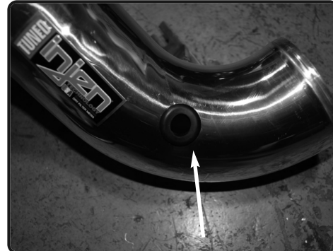
19. Install the grommet to the hole on intake tube. This will be used for temp sensor.
