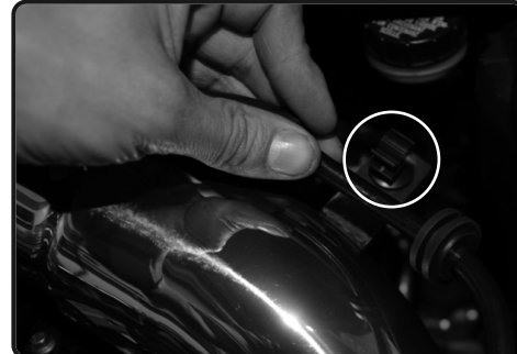
23. Secure the vacuum line to the clip from step 18.
