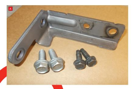
A) The original bolt on support bracket is not required when fitting the Scorpion downpipe. Please remove this with the original downpipe.
